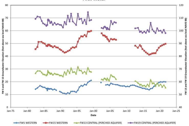
Figure 15 Water Level Hydrographs Perched Aquifer / First Water Los Osos Groundwater Basin 2021 Annual Report
