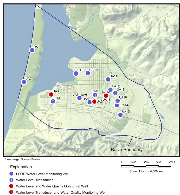
Figure 3 Groundwater Monitoring Program Upper Aquifer Wells Los Osos Groundwater Basin 2021 Annual Report
