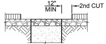
STEP 3: SAWCUT PER NOTE 1 TO REMOVE AN ADDITIONAL 12" MIN OF ASPHALT SURFACE
