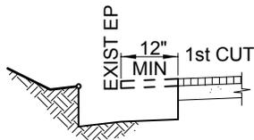
STEP 1: SAWCUT PER NOTE 1 AND REMOVE MATERIAL TO REQUIRED DEPTH.
