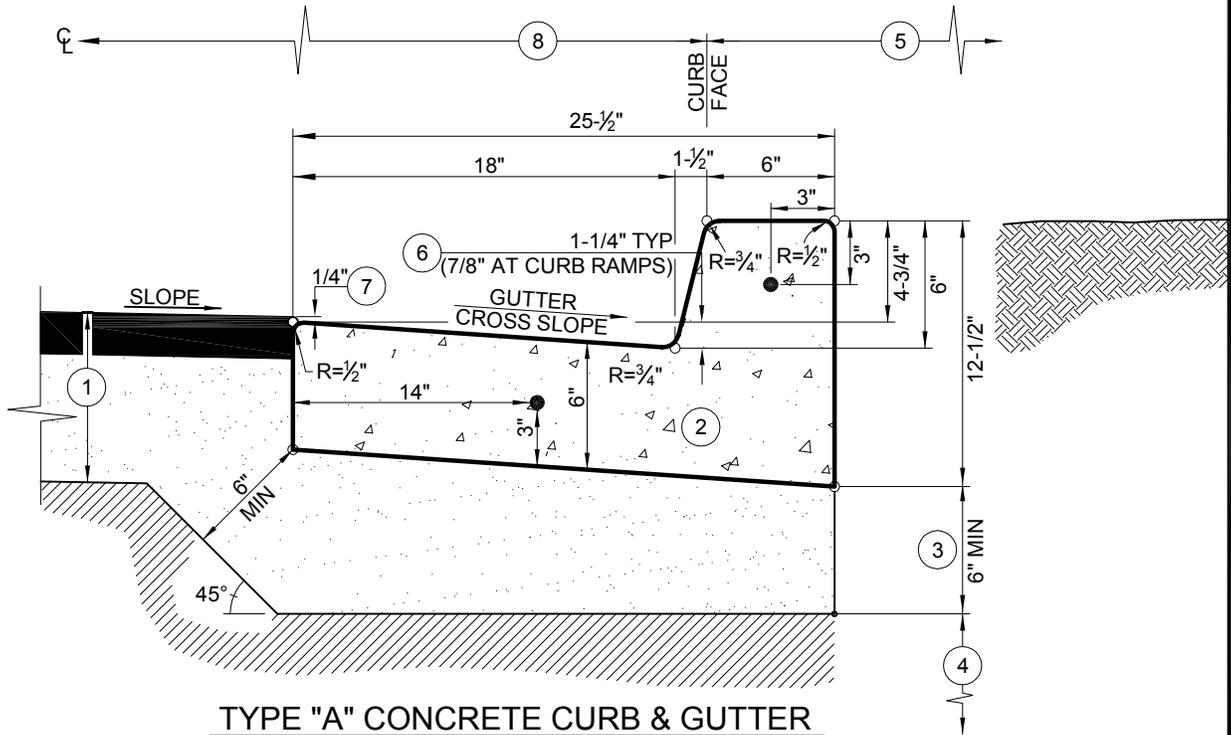
**TYPE "A" CONCRETE CURB & GUTTER**
