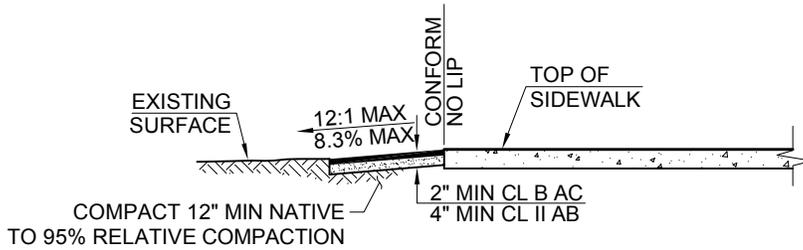
**SECTION A-A: ASPHALT CONCRETE RAMP**
