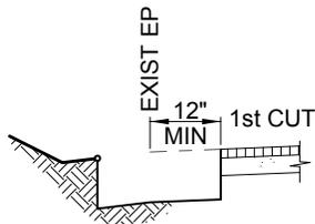
STEP 1: SAWCUT PER NOTE 1 AND REMOVE MATERIAL TO REQUIRED DEPTH.
