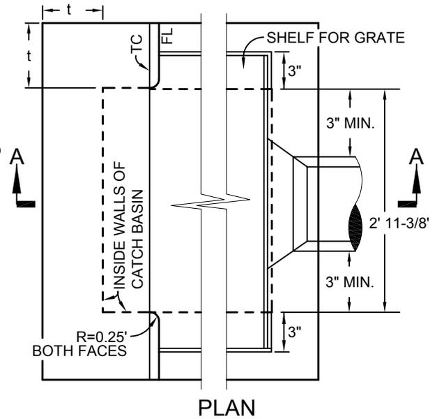
ALL CATCH BASINS SHALL BE EQUIP WITH A STAINLESS STEEL FRAME DESIGNED TO ACCEPT A "DrainPac™" STORM DRAIN FILTER INSERT, OR EQUAL.
