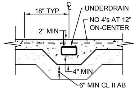
ADD SCORE LINE IN CONCRETE DIRECTLY ABOVE PIPE EDGES
