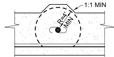
SIDEWALK SHALL BE WIDENED BEHIND ALL ABOVE GRADE OBSTACLES TO PROVIDE A 4-FOOT MINIMUM CLEARANCE.
