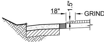
STEP 5: WHEN EXISTING AC IS  $\geq 3.5"$  THICK, GRIND 18" WIDE x 1.5" DEEP OFF EXISTING ASPHALT SURFACE.
