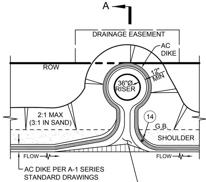
OVERSIDE DRAIN PER STATE STD. D87D (TYPE A OR MOUNTABLE PER PLANS)
