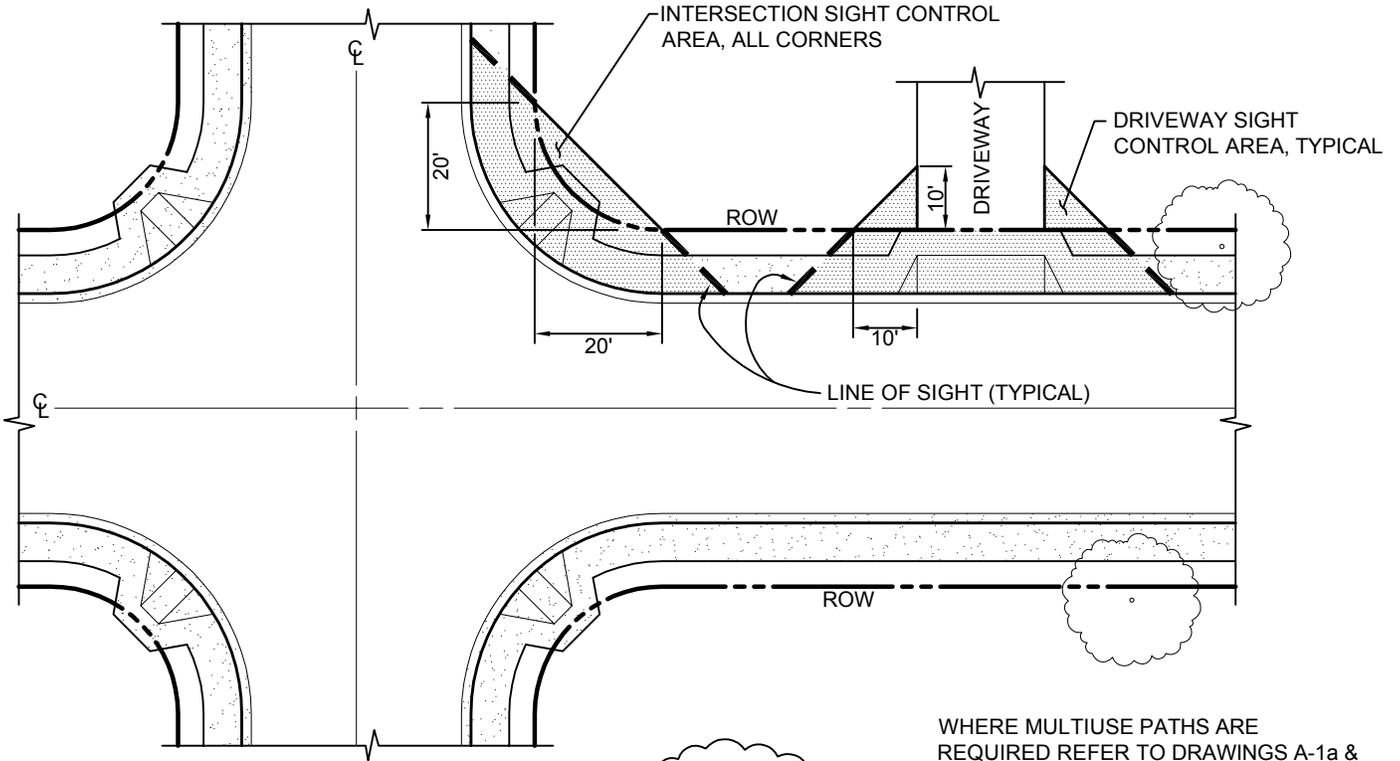
WHERE MULTIUSE PATHS ARE REQUIRED REFER TO DRAWINGS A-1a & A-2a FOR ADDITIONAL CLEARANCE RESTRICTIONS
