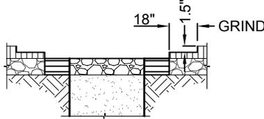
STEP 5: WHEN EXISTING AC IS  $\geq 3.5"$  THICK, GRIND 18" WIDE x 1.5" DEEP OF OFF EXISTING ASPHALT SURFACE.
