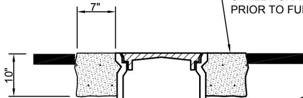
VALVE BOX - BROOKS No. 3RT OR APPROVED EQUAL WITH EXTENSIONS TO VALVE
