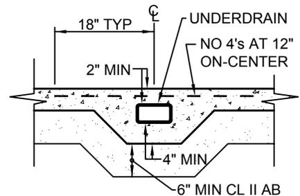
ADD SCORE LINE IN CONCRETE DIRECTLY ABOVE PIPE EDGES
