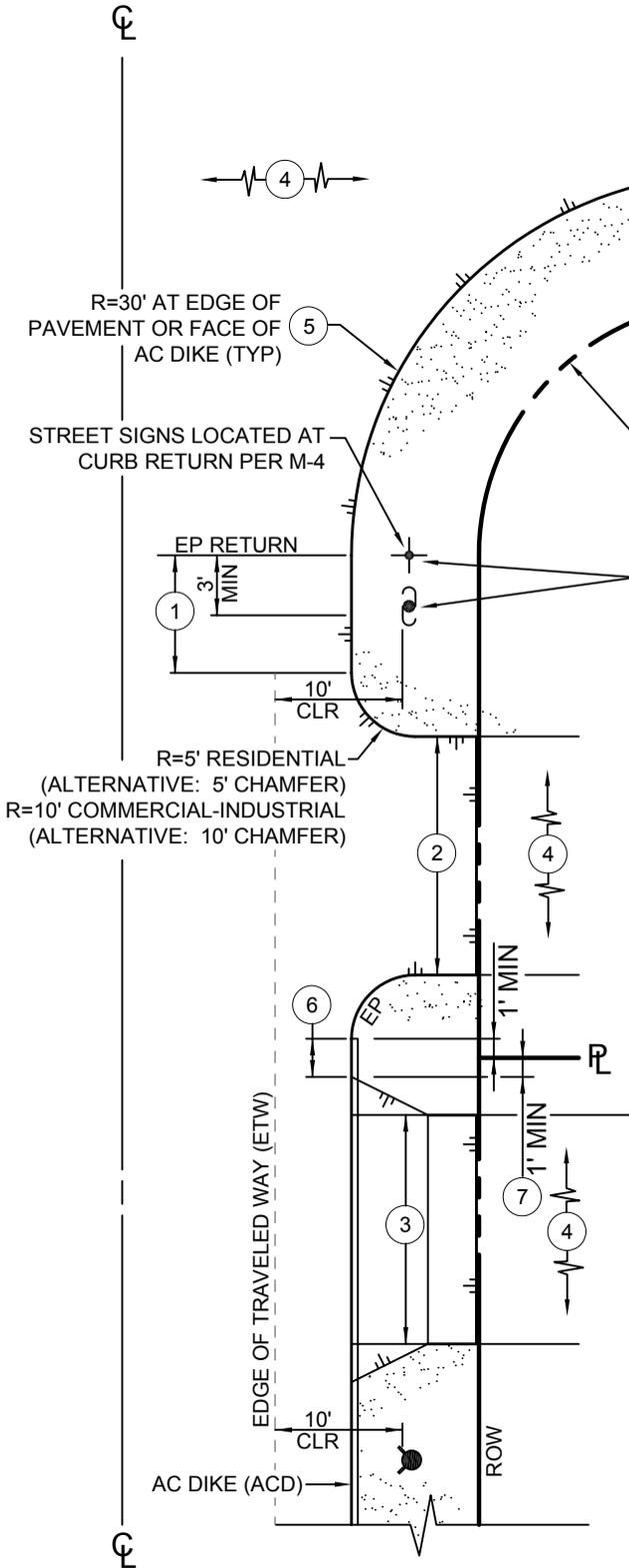
ROAD SIGNS, FIRE HYDRANTS, UTILITY POLES, TRAFFIC SIGNALS, LIGHT STANDARDS, ABOVE GROUND VAULTS AND ALL OTHER ROADSIDE OBSTACLES SHALL BE LOCATED TO PROVIDE A 10-FOOT CLEAR ZONE FROM THE EDGE OF TRAVELED WAY. WITH THE EXCEPTION OF TRAFFIC SIGNS, ALL OBSTACLES SHALL BE LOCATED NO CLOSER THAN 3-FEET TO A RETURN AND SHALL MEET THE SIGHT DISTANCE REQUIREMENTS OF THE A-5 SERIES DRAWINGS.
