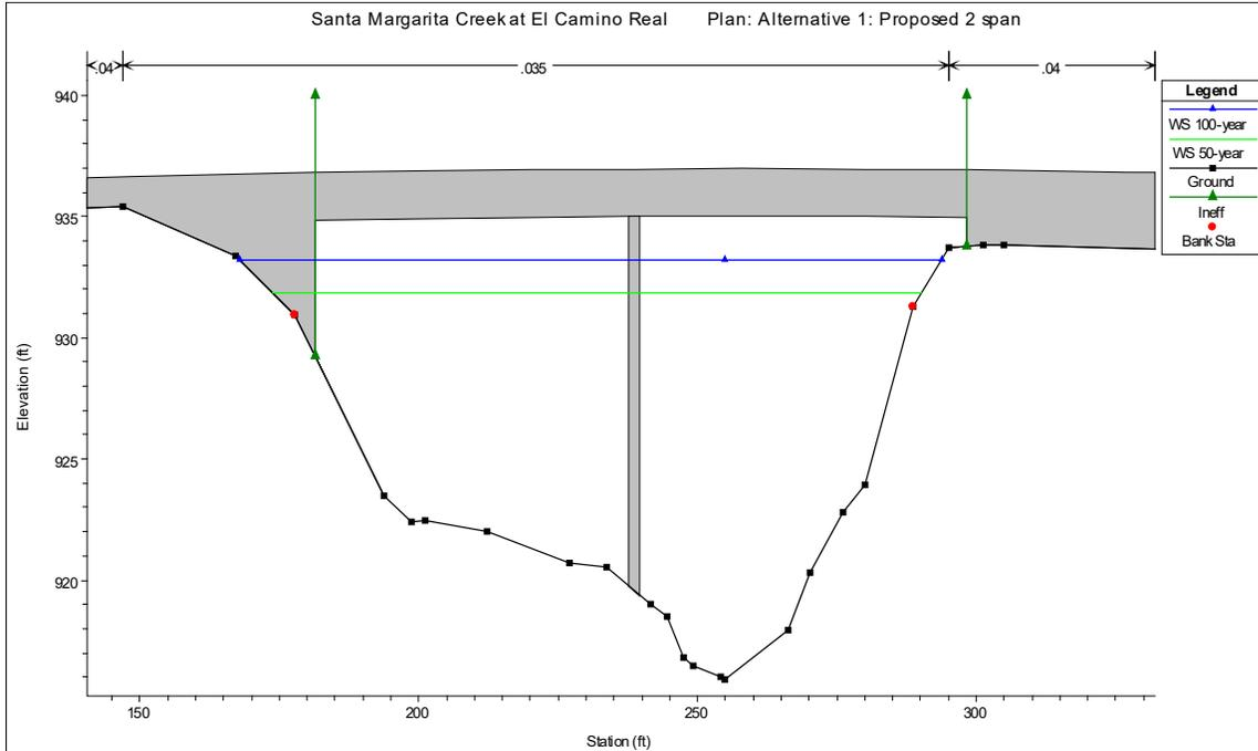
*Figure 1: Alternative 1 – 122 ft, 2-span Bridge*
