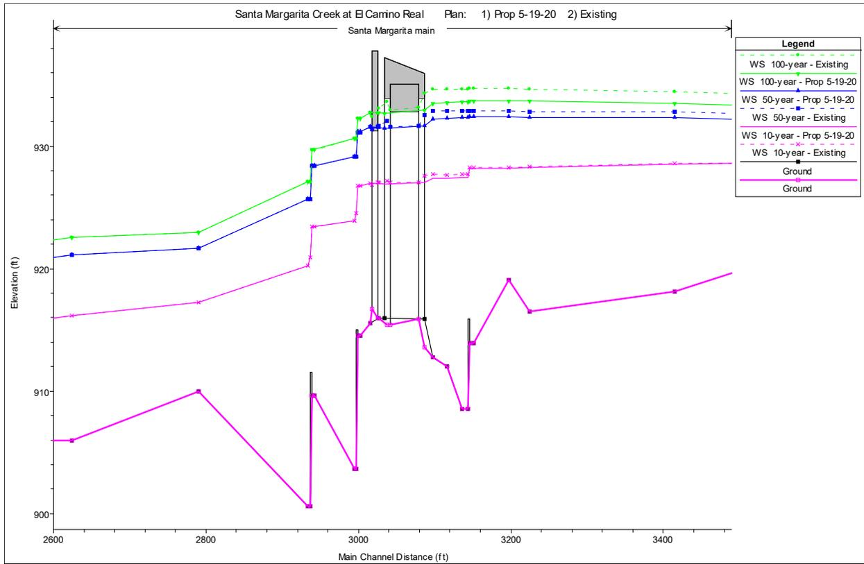
*Figure 9: Water surface elevation comparing Existing vs. Proposed*
