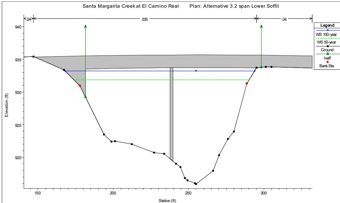
*Figure 3: Alternative 3 – 119 ft, 2-span Bridge*
