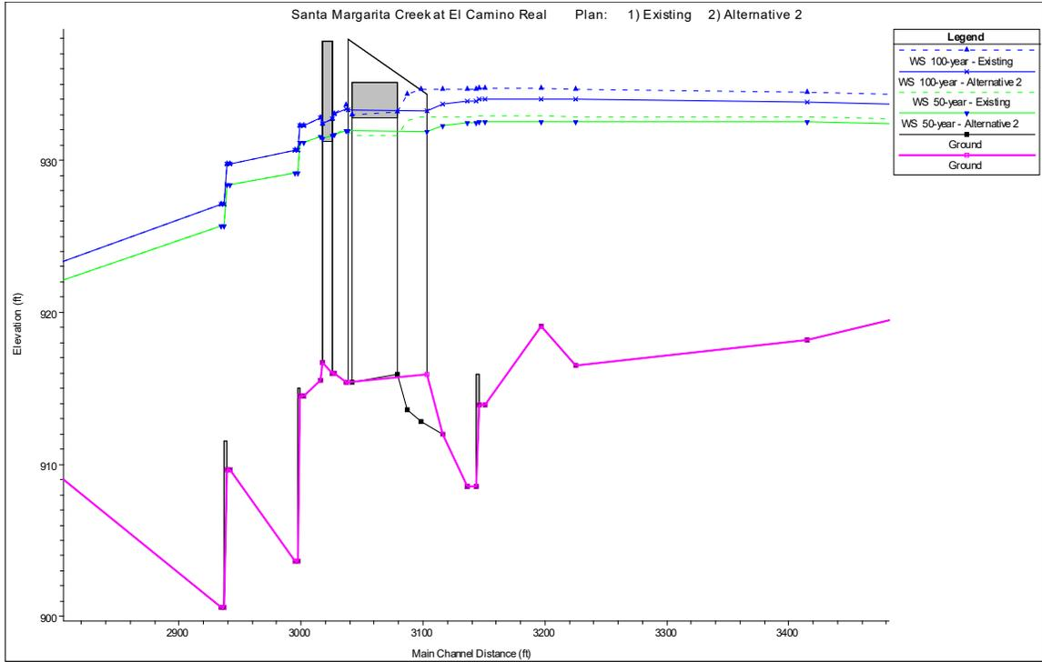
Figure 6: Water surface elevation comparing Existing vs. Alternative 2
