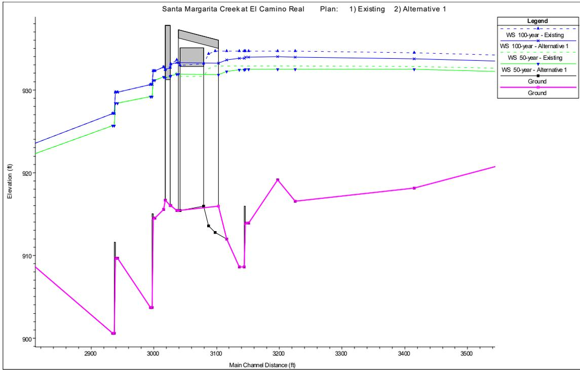
Figure 4: Water surface elevation comparing Existing vs. Alternative 1
