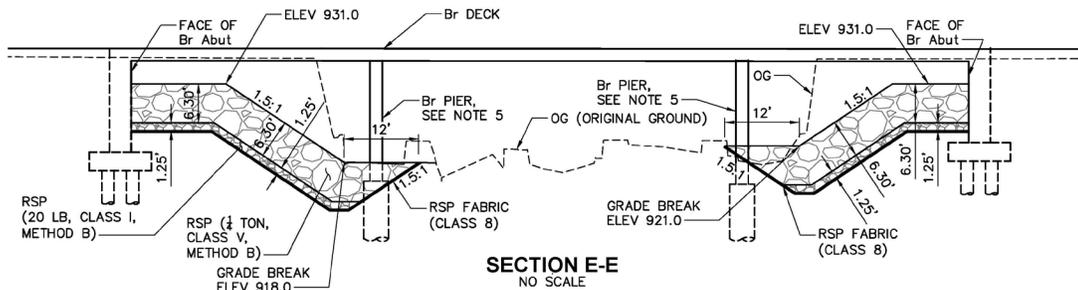
Figure 14: Sections showing RSP under the bridge
