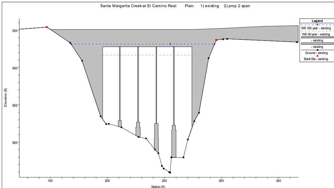
Figure 6: HEC-RAS cross section for the upstream existing conditions for the 50- 100-year  $Q$ 's
