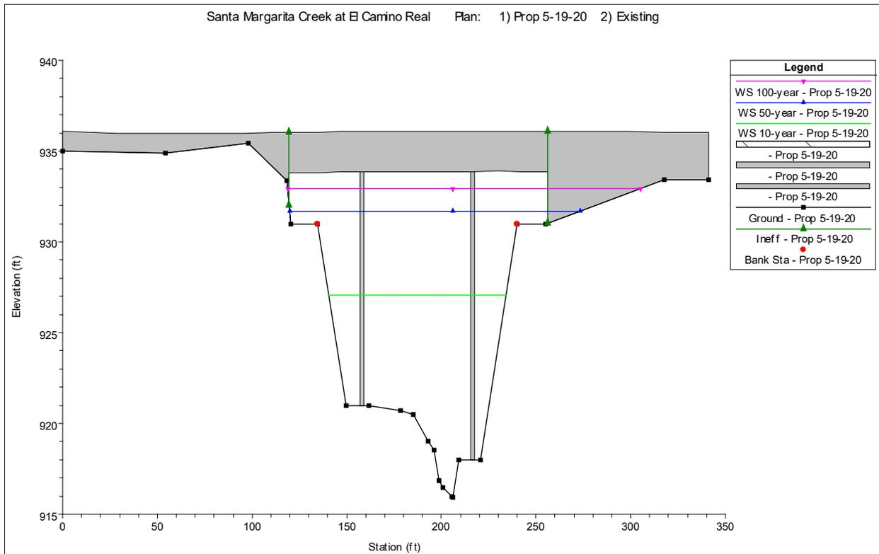
*Figure 8: Proposed 142 ft, 3-span Bridge*
