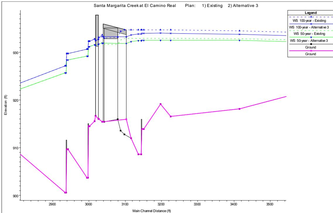
Figure 7: Water surface elevation comparing Existing vs. Alternative 3
