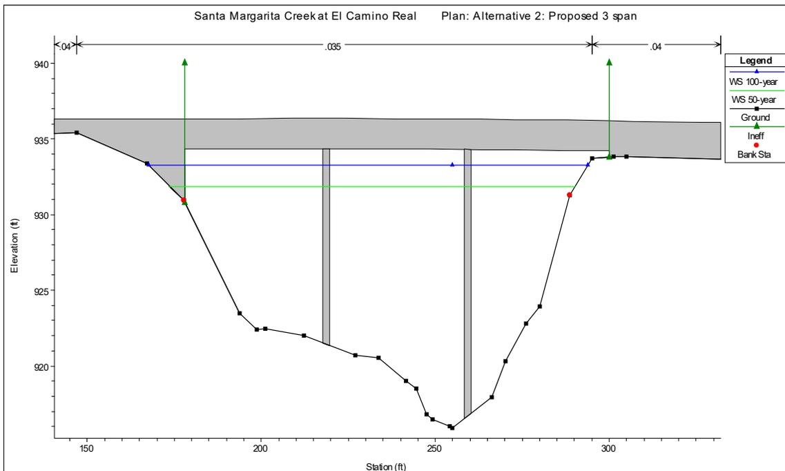
*Figure 2: Alternative 2 – 122 ft, 3-span Bridge*
