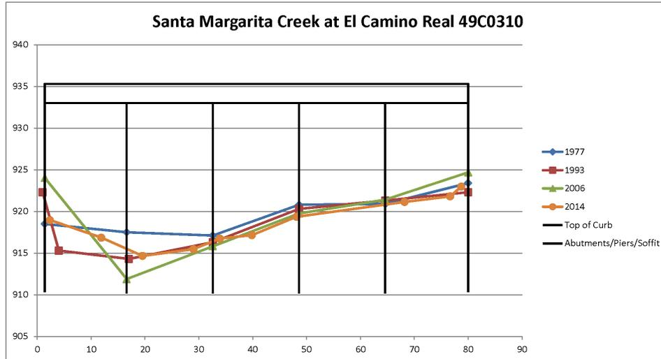
Figure 12: Cross sections taken at the bridge over time (from Caltrans Maintenance Reports)
