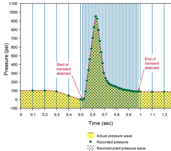
Figure 3 – TP-1 Data Recording Scheme
