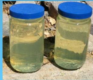
Colloidal sulfur remains in suspension in effluent
