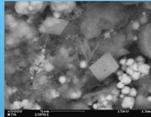
Barite crystals, pyrite (spheres) and Ca-
