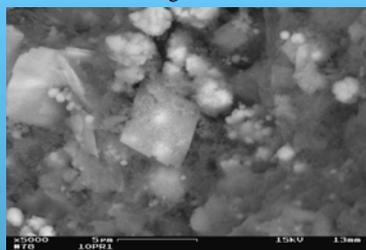
Barite crystals and pyrite (spheres)
