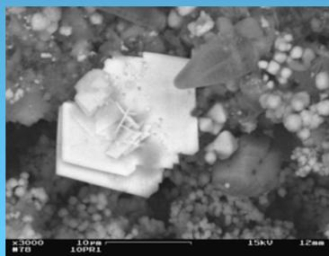
Sulfur crystals (white) and pyrite (spheres)
