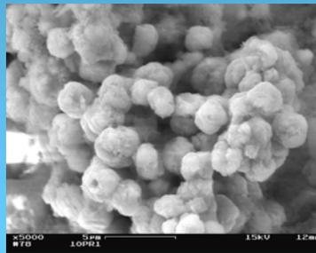
Pyrite (iron sulfide) Spheres
