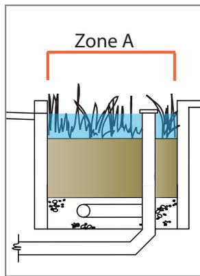
**Uniform surface grade:** This stormwater planter has a flat bottom with consistent depth of ponding across the structure. All of the plants selected for this design must be tolerant of periodic inundation (Zone A).
