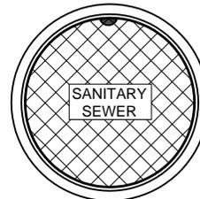
PINKERTON A-640 WITH SKID RESISTANT SURFACE, BLIND PICKHOLE, WATER TIGHT GASKET, AND HS-20 TRAFFIC LOADING, OR APPROVED EQUAL, MARKED "SANITARY SEWER"
