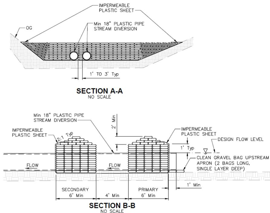
Temporary culverts, consisting of approximately two 18-inch pipes, will be used to divert summer flows away from the work area and downstream. The pipes will be approximately 150' long and will be installed through the upstream and downstream berms running parallel to the direction of flow.
