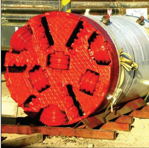
**Figure 7. 54-inch Soltau RVS 600 MTBM.**
