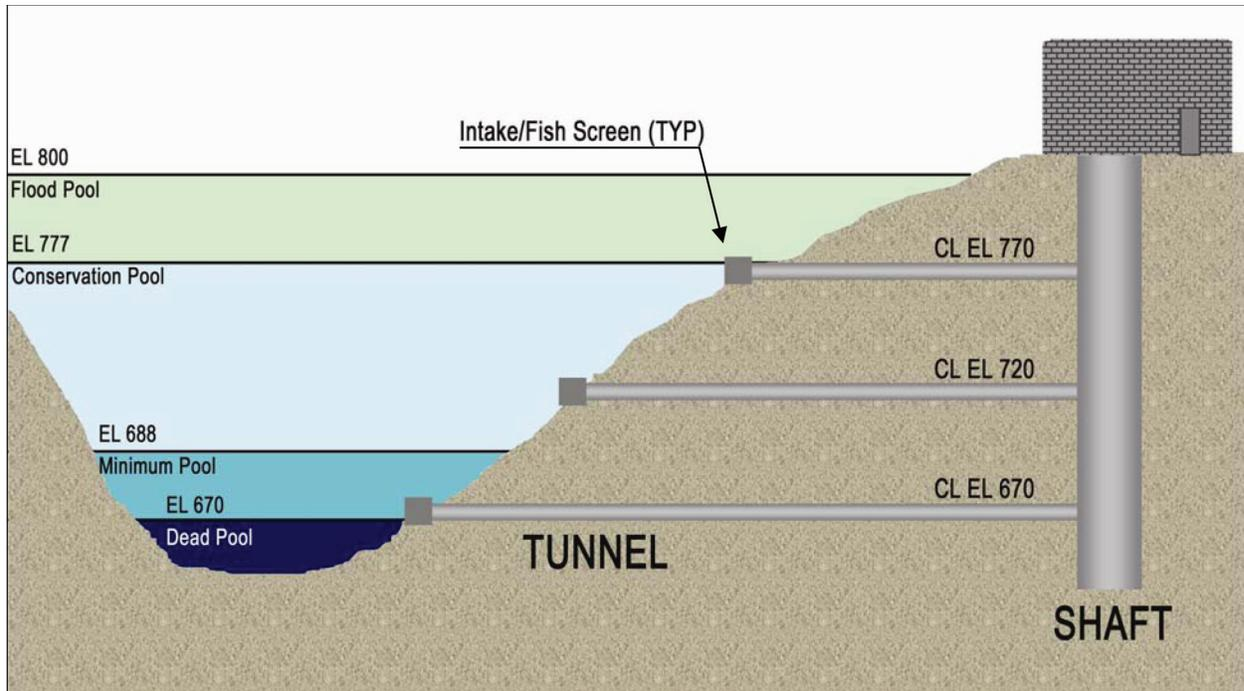
**FIGURE 1. Intake Configuration Presented in Final EIR.**
