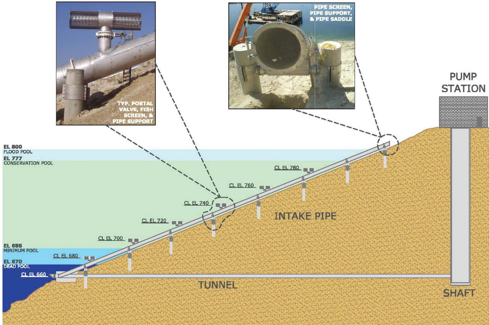
Figure 2. Final Design Configuration of Intake Shaft, Tunnel, and Intake Pipe.
