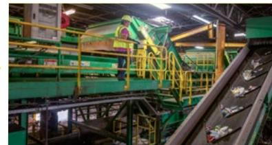
Sortation equipment separates cups, cans, containers and bottles from paper. An eddy current sorts aluminum into a metals-only stream.
