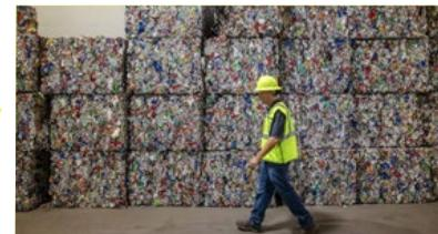
Sorted materials are baled and shipped to customers, where they are used as feedstock for new products.
