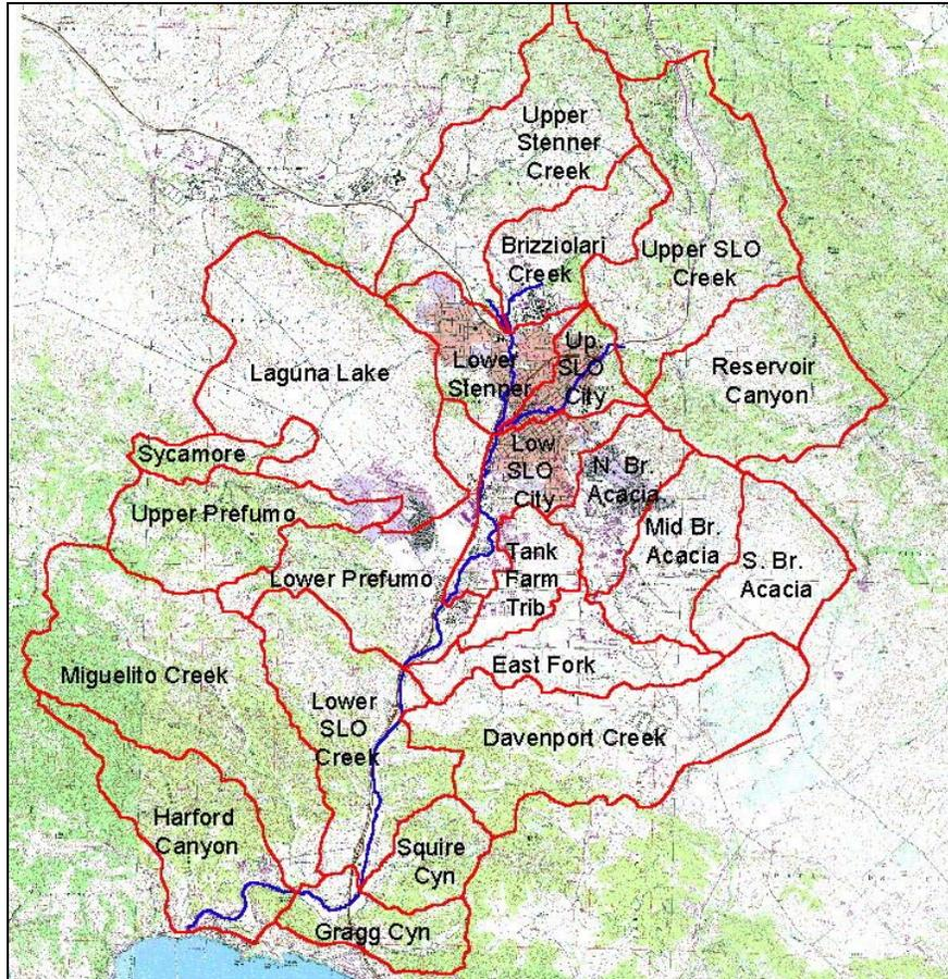
**Figure 1. Hydrology model sub-basin delineation**
