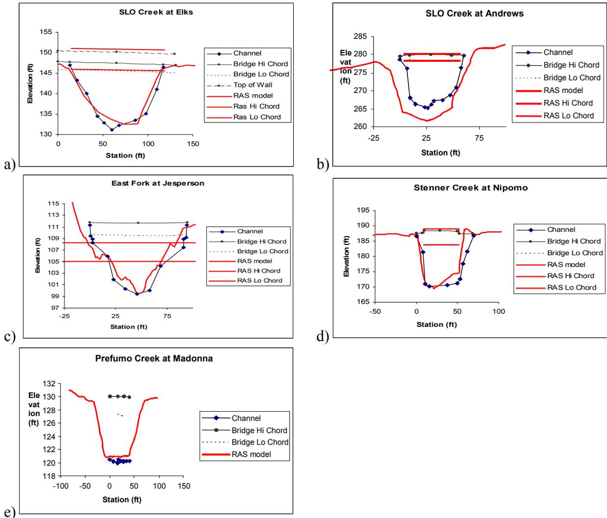
**Figure 5. Cross-sections at County stage gage locations with red lines showing LIDAR data used for the existing hydraulic model and blue lines showing 2006 survey data, which was used to update the hydraulic model: a) Elks Lane Bridge over SLO Creek b) Andrews Street Bridge over SLO Creek c) Jespersion Road Bridge over East Fork of SLO Creek d) Nipomo Street Bridge over Stenner Creek e) Madonna Road Bridge over Prefumo Creek.**
