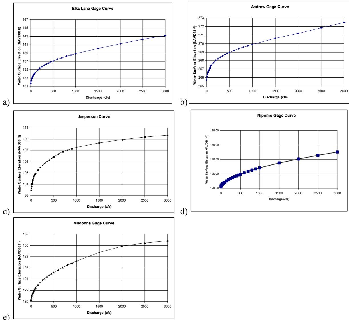
**Figure 6. WSE-discharge curves for County stage gages: a) Elks Lane Bridge over SLO Creek b) Andrews Street Bridge over SLO Creek c) Jespersion Road Bridge over East Fork of SLO Creek d) Nipomo Street Bridge over Stenner Creek e) Madonna Road Bridge over Prefumo Creek.**
