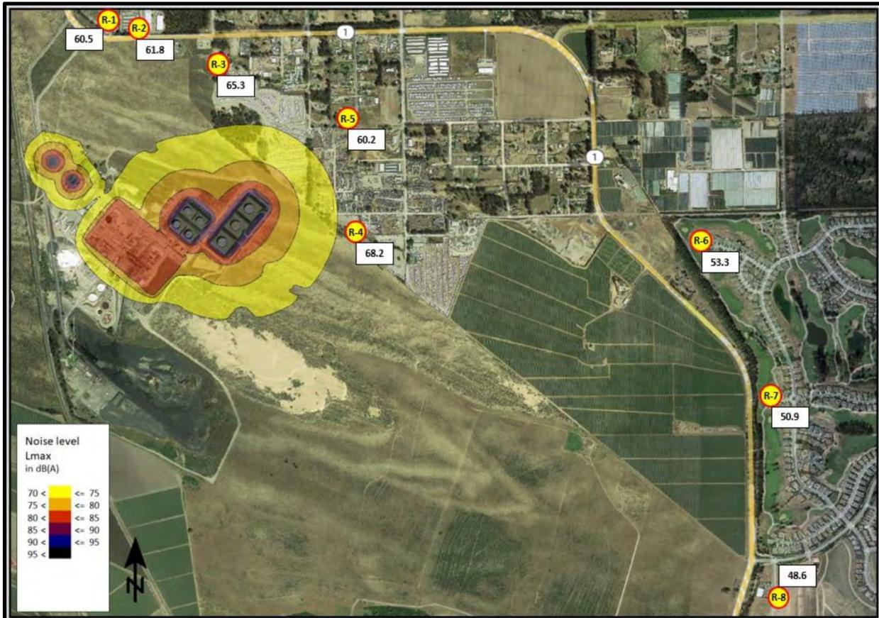
Note: Lmax for single loudest piece of equipment. Noise levels and contours were calculated using the SoundPLAN<sup>®</sup> computer program assuming receiver would be placed at a height of approximately five feet above ground level. Locations are approximate.
