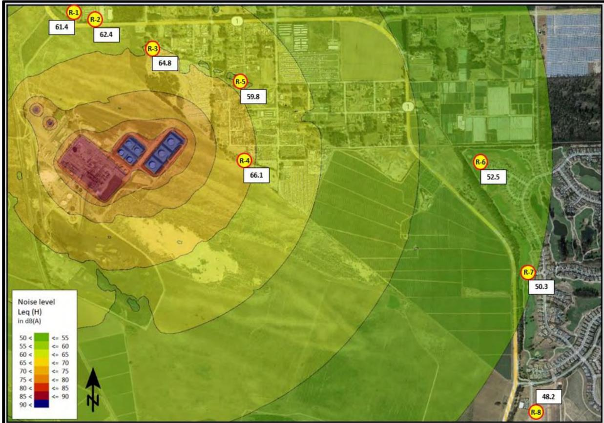
Note: Noise levels and contours were calculated using the SoundPLAN<sup>®</sup> computer program assuming receiver would be placed at a height of approximately five feet above ground level. Locations are approximate.
