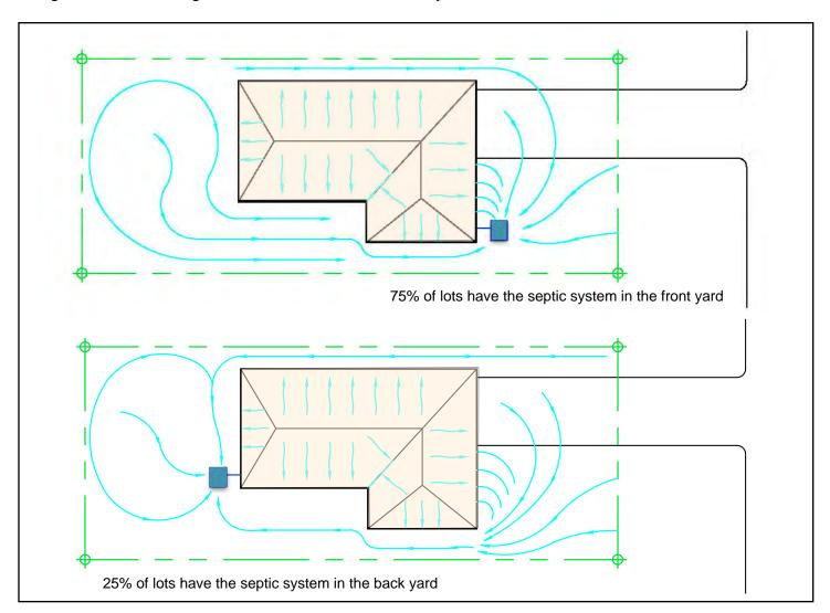
Above: The light blue water flow arrows direct rainwater and stormwater to the former septic system to accomplish the Low Impact Development (LID) objective.
