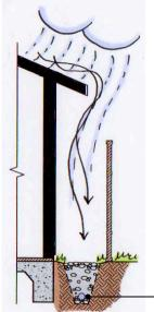
French Drain: a walkable gravel surface with underground perforated drain pipe, sloping toward front yard, encased in a gravel filled trench to take water toward front yard and into the tank system. This approach may take additional maintenance if piping becomes clogged.
