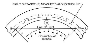
HEIGHT OF EYE = 3.50. HEIGHT OF OBJECT = 0.50 FEET LINE OF SIGHT IS 2.0 FEET ABOVE  $\[ \varphi \]$  INSIDE LANE AT POINT OF OBSTRUCTION.
