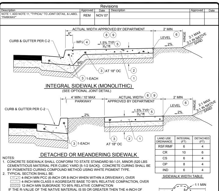
AGGREGATE BASE MAY BE SUBSTITUTED WITH COMPACTED NATIVE MATERIAL.
