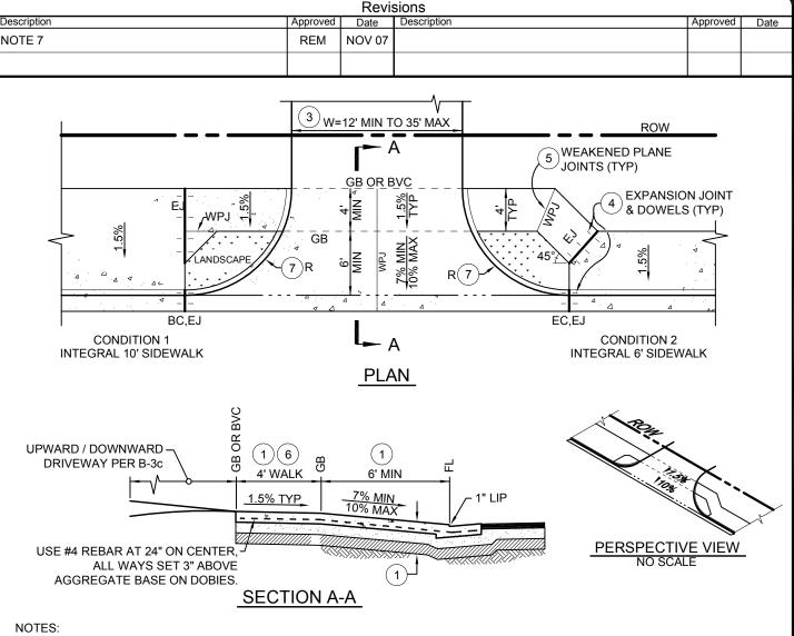
CONCRETE DRIVEWAY SHALL CONFORM TO STATE STANDARD 90-1.01, 520 LBS/CY CEMENTITIOUS MATERIAL [5-1/2 SACK]. CONCRETE CURING SHALL BE BY PIGMENTED CURING COMPOUND METHOD USING WHITE PIGMENT TYPE. TYPICAL SECTION SHALL BE:
