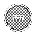
PINKERTON A-640 WITH SKID RESISTANT SURFACE, BLIND PICKHOLE, WATER TIGHT GASKET, AND HS-20 TRAFFIC LOADING, OR APPROVED EQUAL, MARKED "SANITARY SEWER"
