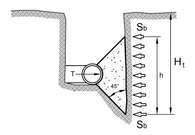
THE REQUIRED BEARING BLOCK AREA IS  $A_b = hb = \frac{Sf T}{S_b}$
