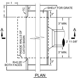
ALL CATCH BASINS SHALL BE EQUIP WITH A STAINLESS STEEL FRAME DESIGNED TO ACCEPT A 'DrainPac™" STORM DRAIN FILTER INSERT, OR EQUAL
