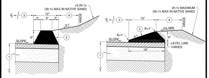
TYPE "A" HMA DIKE FOR USE IN CUT CONDITIONS > 2.5:1
