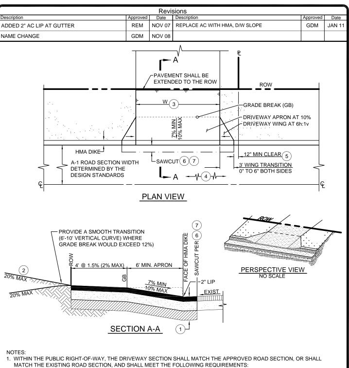
HOT MIX ASPHALT (HMA) PER THE DESIGN STANDARDS TO 95% RELATIVE COMPACTION, OVER CLASS II AGGREGATE BASE TO 95% RELATIVE COMPACTION, OVER
