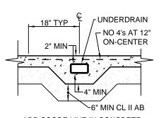
ADD SCORE LINE IN CONCRETE DIRECTLY ABOVE PIPE EDGES
