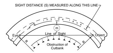
HEIGHT OF EYE = 3.50. HEIGHT OF OBJECT = 0.50 FEET LINE OF SIGHT IS 2.0 FEET ABOVE  $\mbox{\ensuremath{\mathbb{Q}}}$  INSIDE LANE AT POINT OF OBSTRUCTION.
