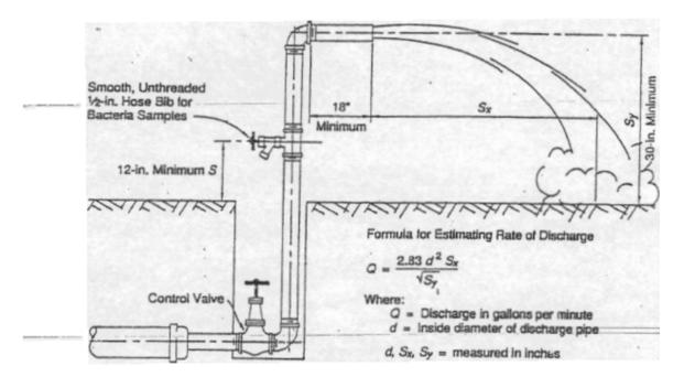
NOTE: This figure applies to pipes up to and including 8-in. (200 mm) diameter.
