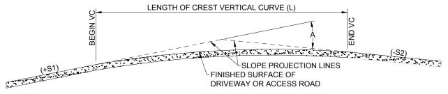
FIG 1: CREST VERTICAL CURVE
