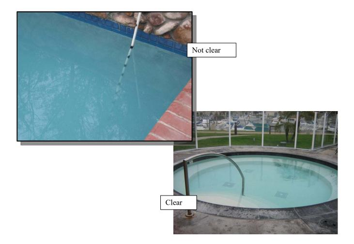
**SAFETY TIP!** Check daily to see if you can easily see the main drain covers from the deck. If the drain is not visible, close the pool until the water clarity
