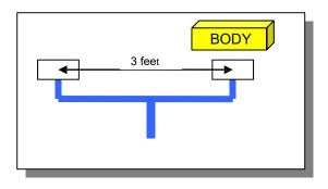
• <u>Secondary layer of protection is required if the pool has a single blockable drain or has</u> multiple drains less than 3 feet apart. Secondary layers of protection include:
