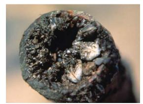
QMs clog pipes and intake structures causing severe damage that requires heavy annual maintenance
