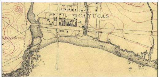
**Figure 7.** U.S. Coast & Geodetic Survey T-sheet, Image # T1663-00-1884. Not surprising in a nautical map, the details focus on the wharf configuration, character of the coastline, and nearshore topography — but the warehouse, lumber shed, and water tank are also clearly indicated.
