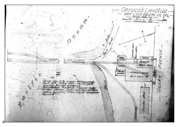
*Figure 8.* Plan view of warehouses and wharf at Cayucos Landing, November 1885, from Dakin's *California Warehouse Book*. Dakin's maps, like Sanborn maps, were intended for insurance underwriting purposes. Here, the interior spaces of the warehouse building are clearly defined, as well as the tramways running from both the main warehouse room and the general merchandise store occupying one corner. The one-story shed-roof addition on the northwest side was also used for merchandise.
