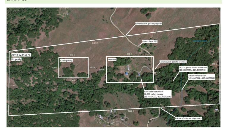
This example of a property diagram used aerial imagery and a basic image-editing software program to accurately label each property diagram requirement.
