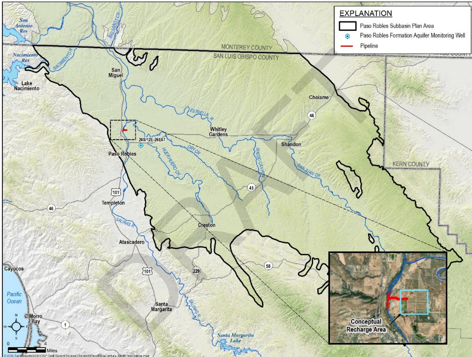
Figure 9-34. Conceptual Flood Flow Capture and Recharge North of City of Paso Robles Project Layout
