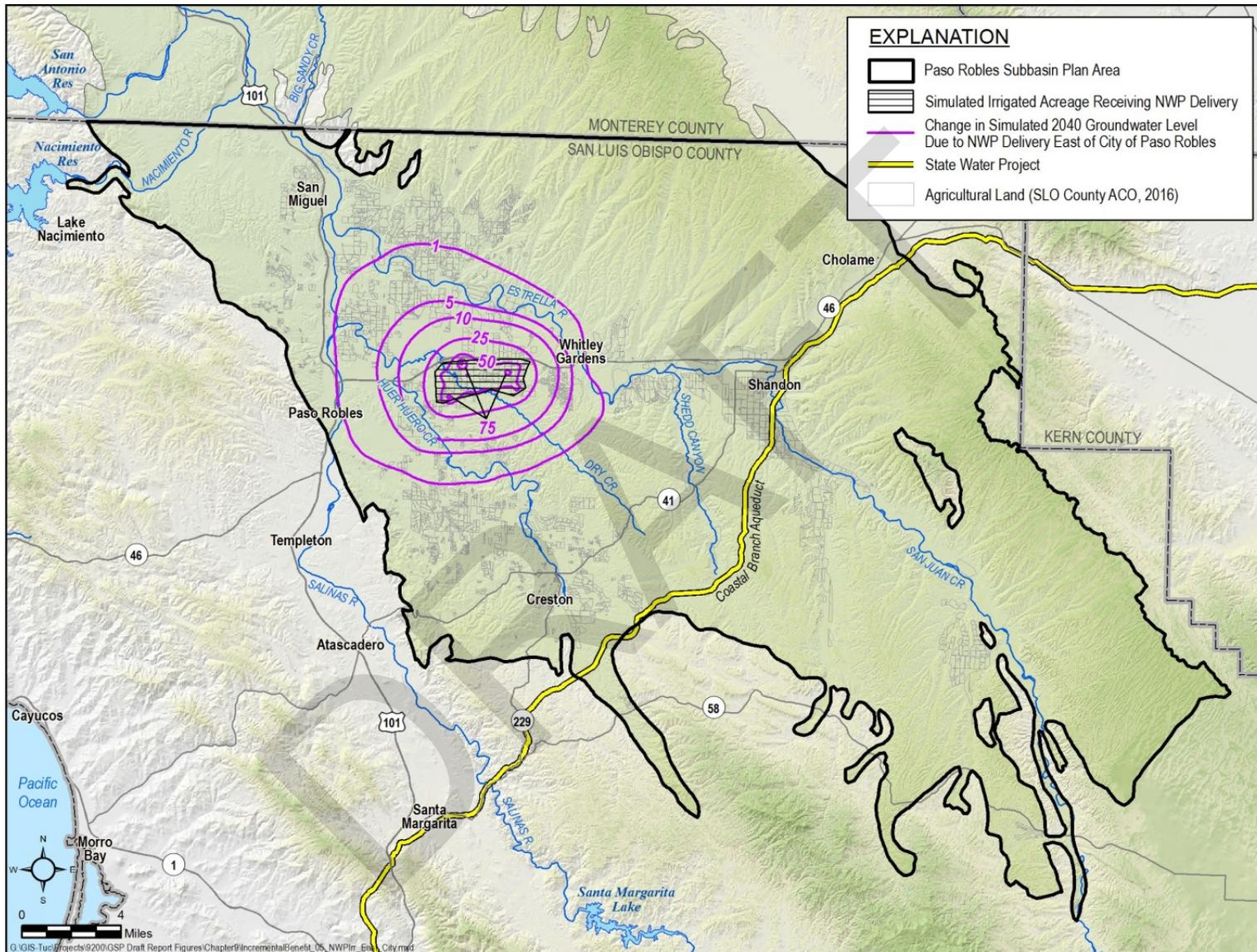
Figure 9-21. Groundwater Level Benefit from NWP Delivery East of City of Paso Robles
