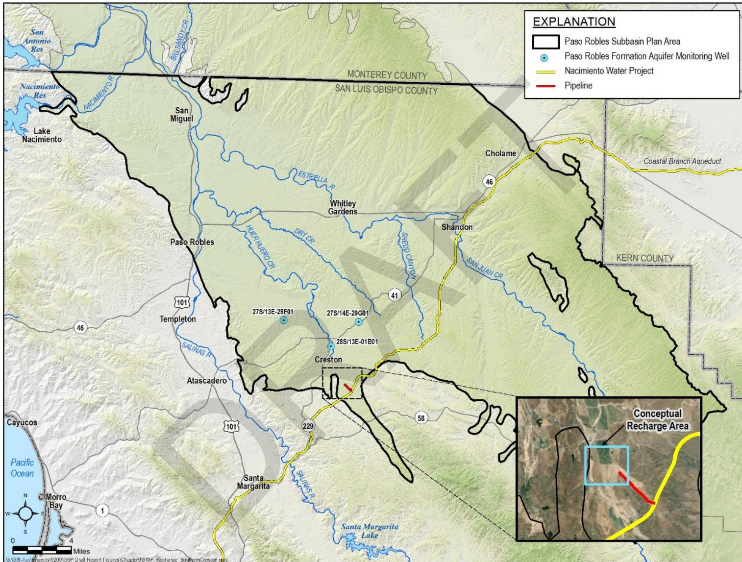
Figure 9-25. Conceptual Recharge Basin in Southwestern Subbasin Project Layout
