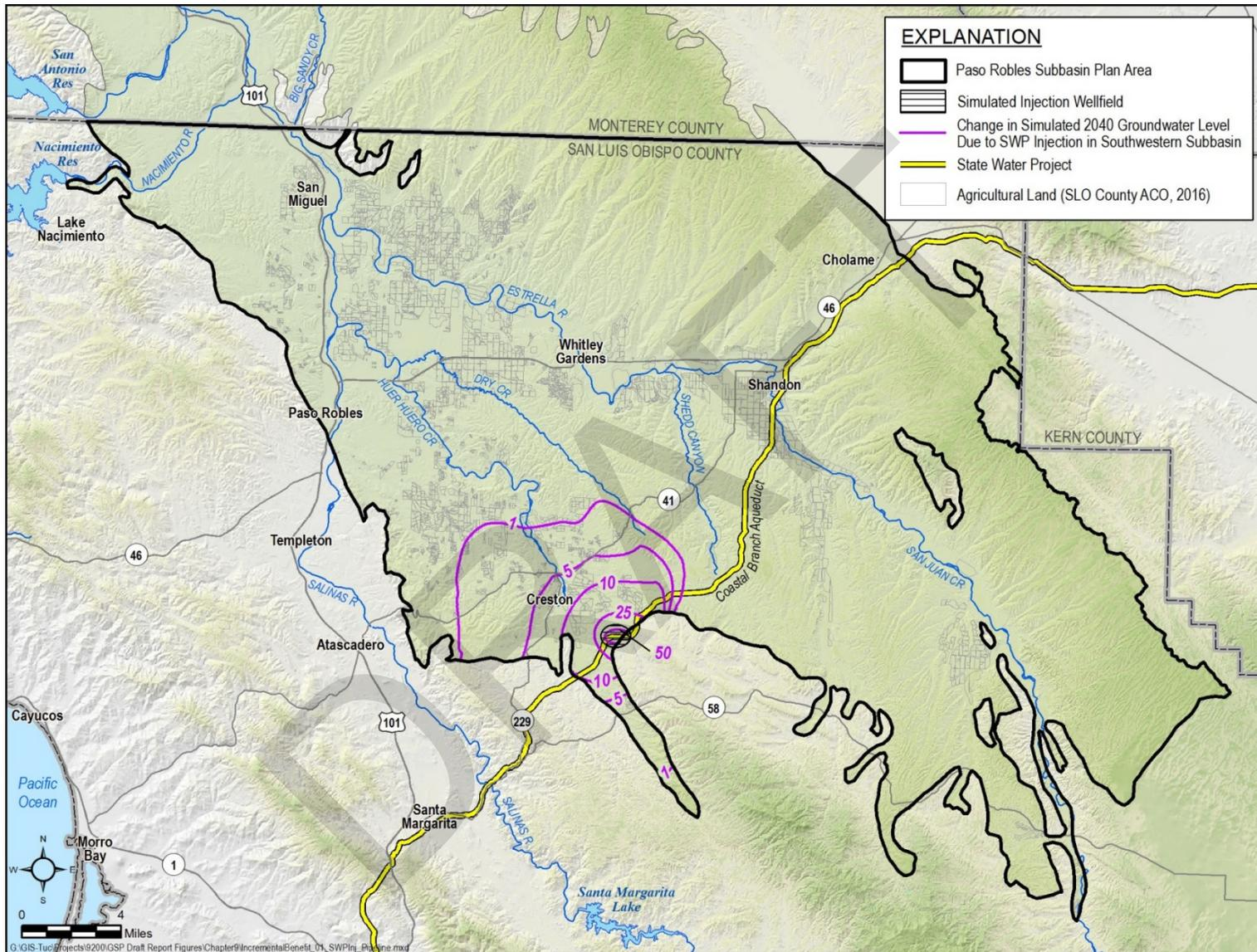
Figure 9-9. Groundwater Level Benefit of SWP Injection in Southwestern Subbasin
