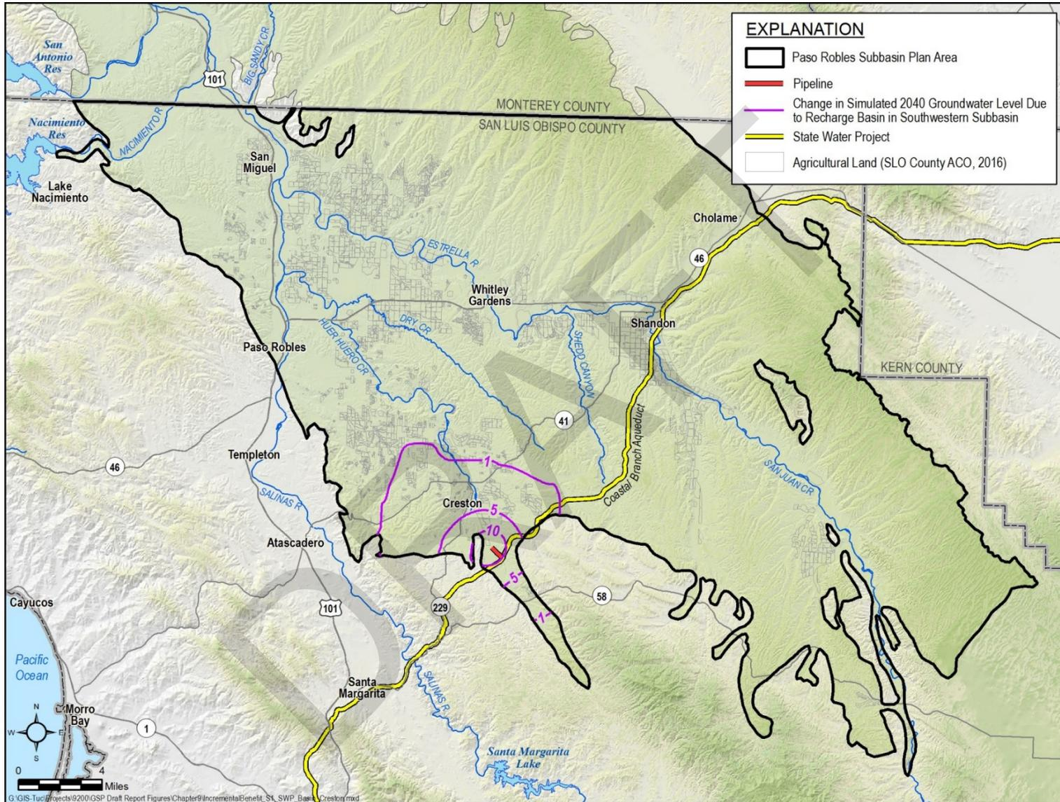
Figure 9-26. Groundwater Level Benefit from Recharge Basin in Southwestern Subbasin
