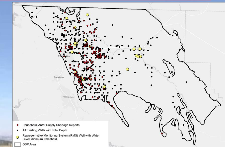
Well location accuracy limits our ability to interpolate MT surface at existing well locations
