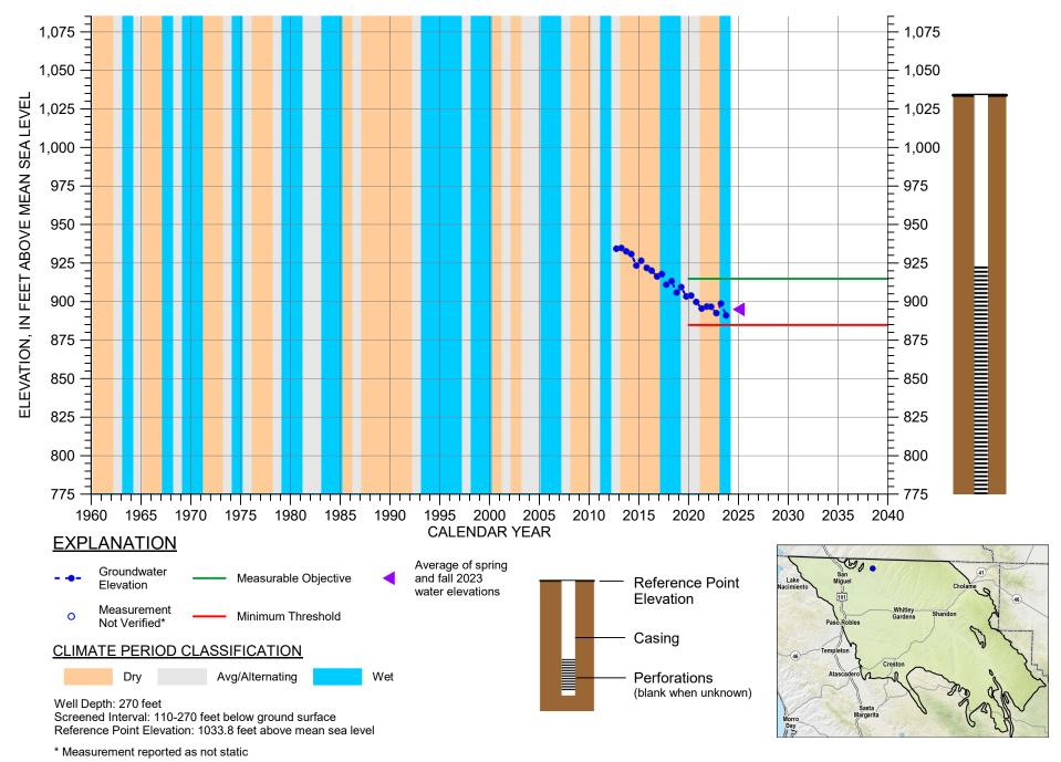
HYDROGRAPH OF MEASURED GROUNDWATER ELEVATION FOR 25S/13E-08L02
