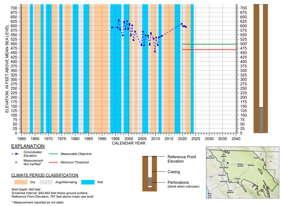
HYDROGRAPH OF MEASURED GROUNDWATER ELEVATION FOR 26S/12E-14G02
