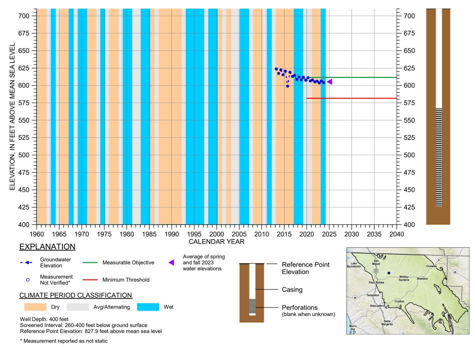
HYDROGRAPH OF MEASURED GROUNDWATER ELEVATION FOR 26S/13E-08M01
