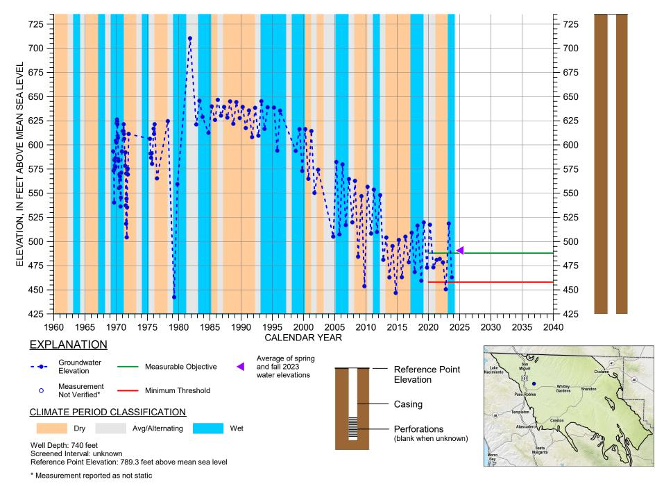
HYDROGRAPH OF MEASURED GROUNDWATER ELEVATION FOR 26S/12E-14G01
