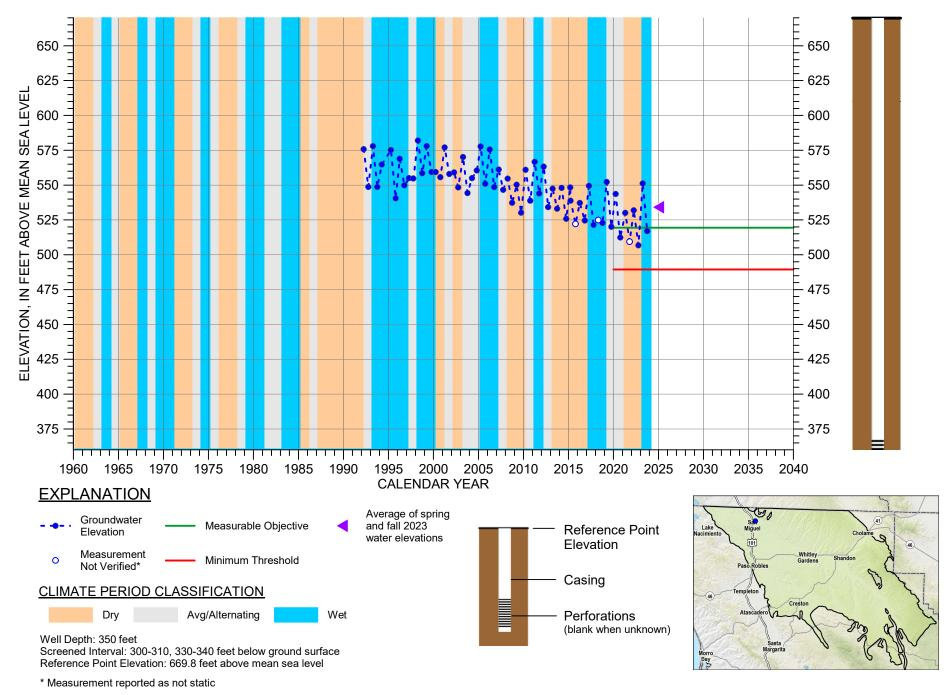
HYDROGRAPH OF MEASURED GROUNDWATER ELEVATION FOR 25S/12E-16K05
