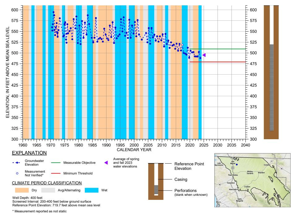
HYDROGRAPH OF MEASURED GROUNDWATER ELEVATION FOR 25S/12E-26L01
