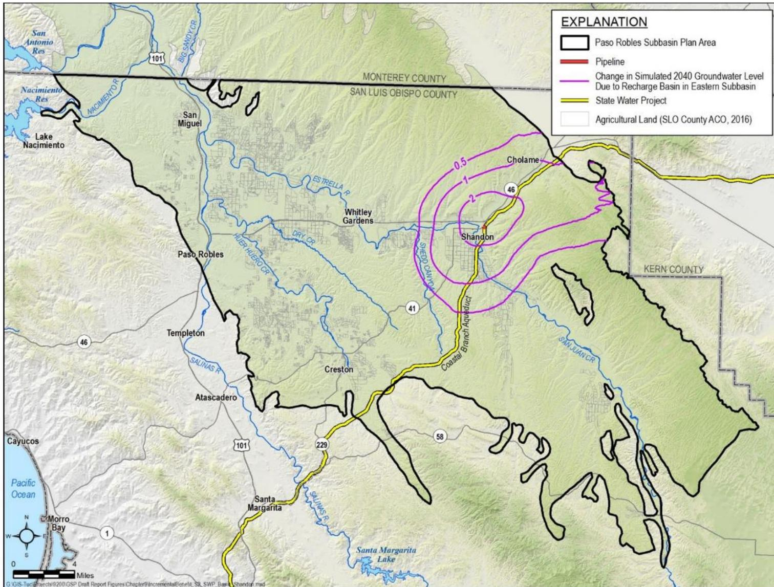
Figure 9-23. Groundwater Level Benefit from Recharge Basin in Eastern Subbasin
