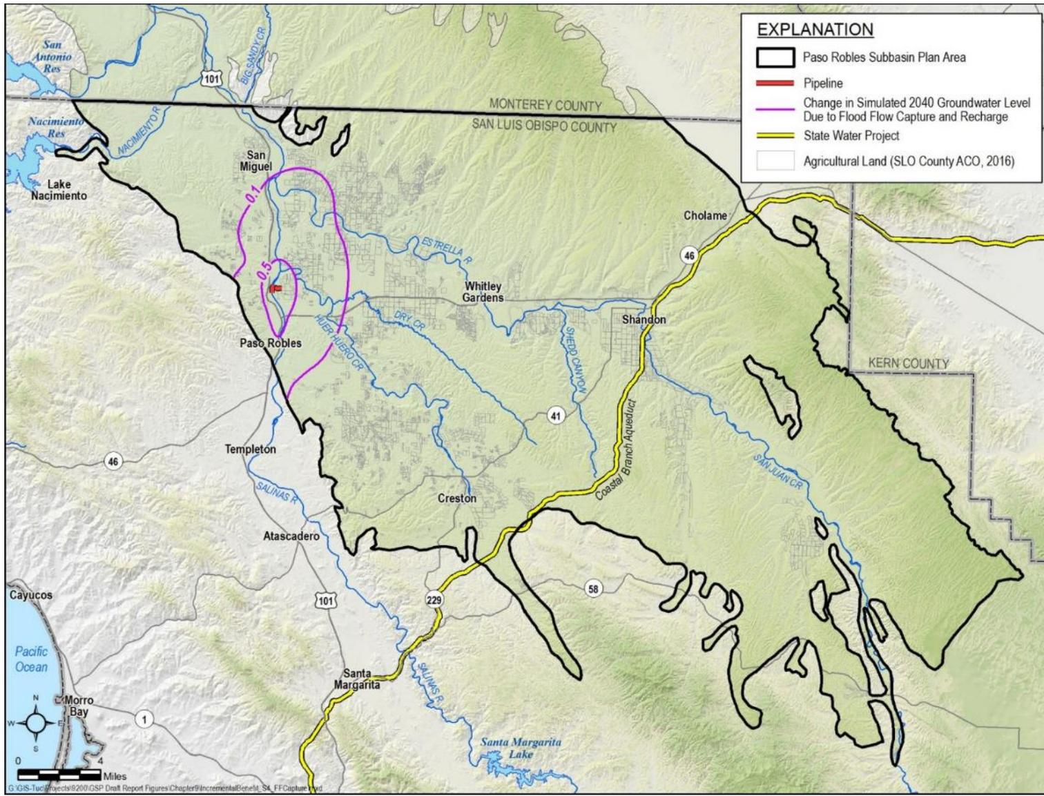
Figure 9-29. Groundwater Level Benefit from Flood Flow Capture and Recharge North of City of Paso Robles
