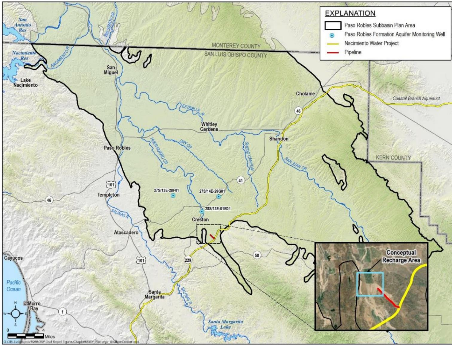
Figure 9-19. Conceptual Recharge Basin in Southwestern Subbasin Project Layout
