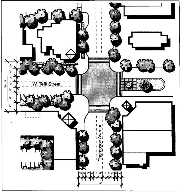
Figure 3.6 Intersection with Speed Table
