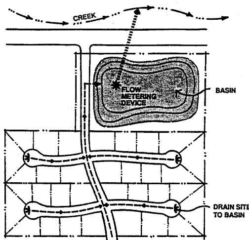
THE PRIMARY FUNCTION OF A DETENTION BASIN IS TO CONTROL THE RATE AT WHICH STORM WATER IS RELEASED FROM A DEVELOPMENT SITE. IN TEMPLETON, DETENTION IN THE UPPER REACHES OF TOAD CREEK WILL HELP TO PREVENT FLOODING IN THE LOWER REACHES. BASINS CAN PROVIDE DUAL USE FACILITIES: CAN BE USED FOR PARKS, BALLFIELDS OR OPEN SPACE.
