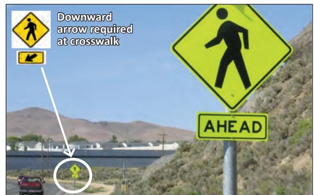
Pedestrian warning signs alert motorists when approaching locations where pedestrian crossing activity is unexpected or not readily apparent. Pedestrian crossing signs at crosswalks require a downward arrow beneath the sign pointing to the marked crosswalk. Flashing amber lights can be added to signs to increase visibility.
