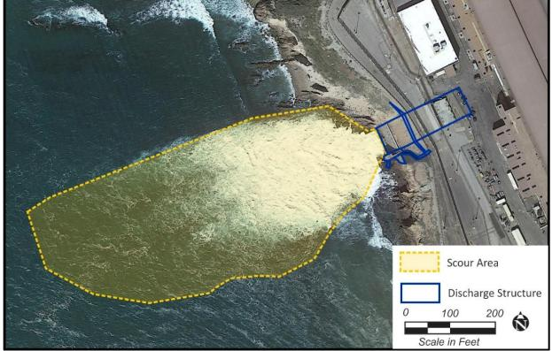
Figure 2-19. Plan View of Existing Discharge Structure and Scour Area
