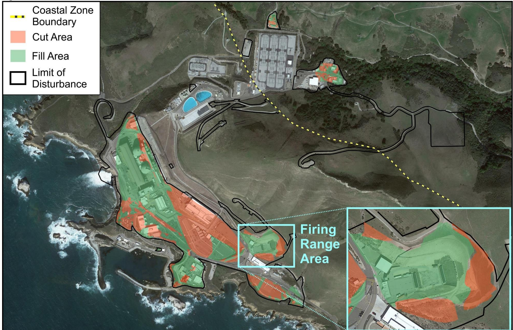
Figure 5-10. Alternative 5 – Partial Backfill
