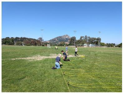
Electrodes are all connected by cables to a central unit that controls the survey.
