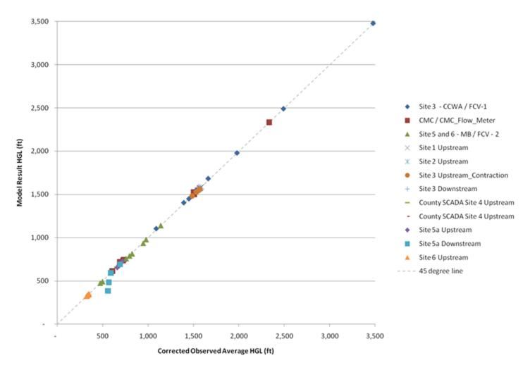
Figure 6-2. Chorro Valley pipeline model calibration correlation plot
