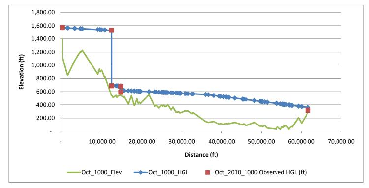
Figure 2. Chorro Valley pipeline hydraulic profile for a flow rate to Morro Bay of 980 gpm.
