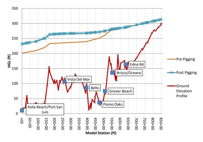
Figure 4. HGL Comparison (Pre/Post Pigging) at Scenario A flow rates
