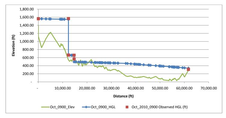
Figure 1. Chorro Valley pipeline hydraulic profile for a flow rate to Morro Bay of 760 gpm.
