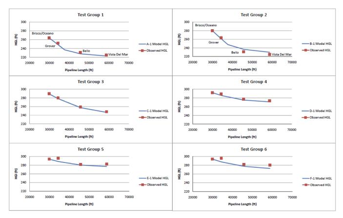
Figure 2. Lopez Pipeline Model - Calibration Profile Plots
