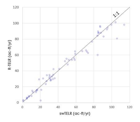
**Figure 3C-7.** Validation experiment results comparing swTELR outputs with those of R-TELR for 63 urban catchments within the City of Watsonville.
