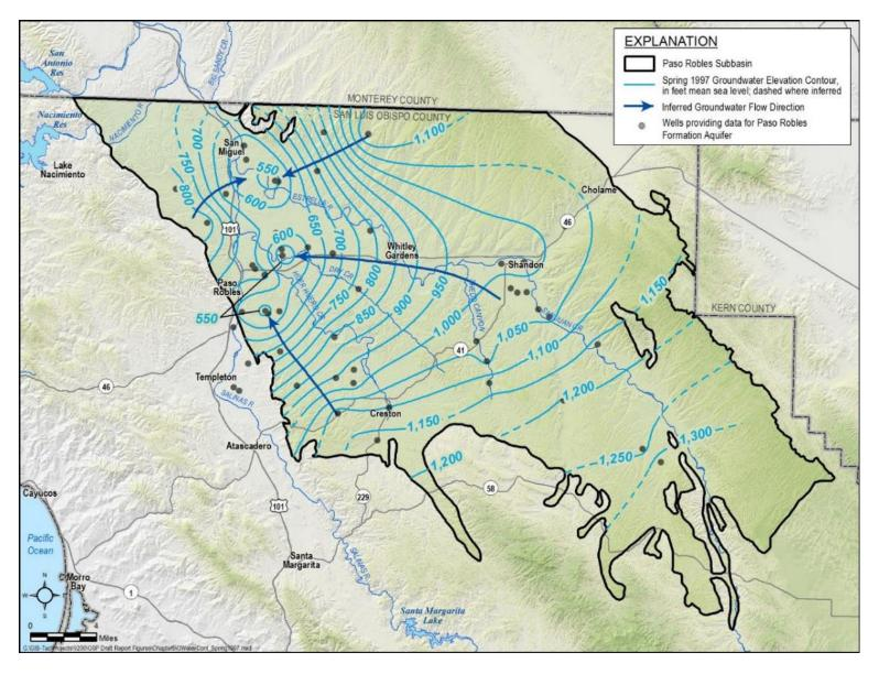
Figure 5-3. Paso Robles Formation Aquifer Spring 1997 Groundwater Elevation Contours
