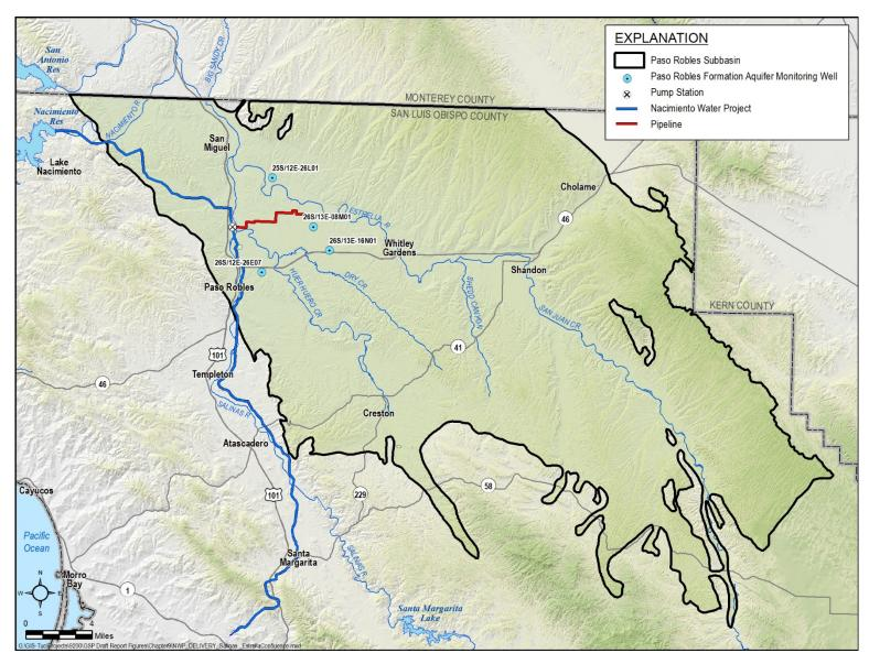
Figure 9-11. Conceptual NWP Delivery North of City of Paso Robles Project Layout
