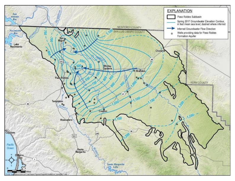
Figure 5-5. Paso Robles Formation Aquifer Spring 2017 Groundwater Elevation Contours
