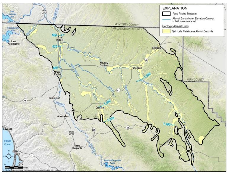
Figure 5-2. Groundwater Elevation Contours for the Alluvial Aquifer
