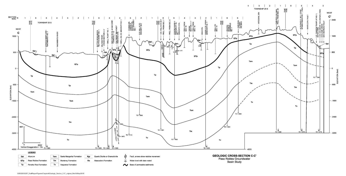
Figure 4-8. Geologic Section C-C'
