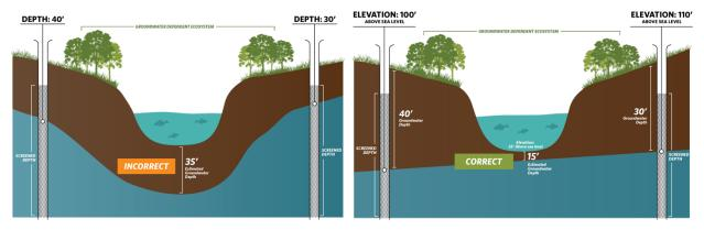
**Figure 6. Contouring depth to groundwater around surface water features and GDEs. (Left)** Groundwater level interpolation using depth to groundwater data from monitoring wells. **(Right)** Groundwater level interpolation using groundwater elevation data from monitoring wells and DEM data.
