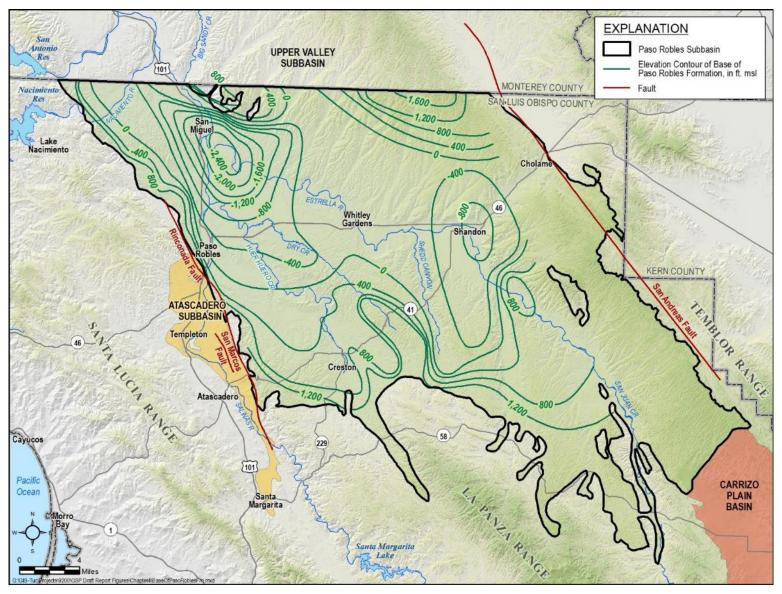
Figure 4-2. Base of Subbasin as Defined by the Base of the Paso Robles Formation
