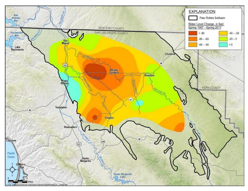
Figure 5-7. Paso Robles Formation Aquifer Change in Groundwater Elevation – Spring 1997 to Spring 2017
