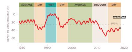
Figure 3. Example seasonality and interannual variability in depth-to-groundwater time. Selecting one point in time, such as Spring 2018, groundwater characterize conditions in GDEs fails to capture what groundwater conditions are necessary to maintain the ecosystem status into the future so adverse impacts are avoided.
