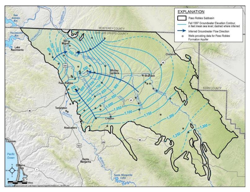
Figure 5-4. Paso Robles Formation Aquifer Fall 1997 Groundwater Elevation Contours
