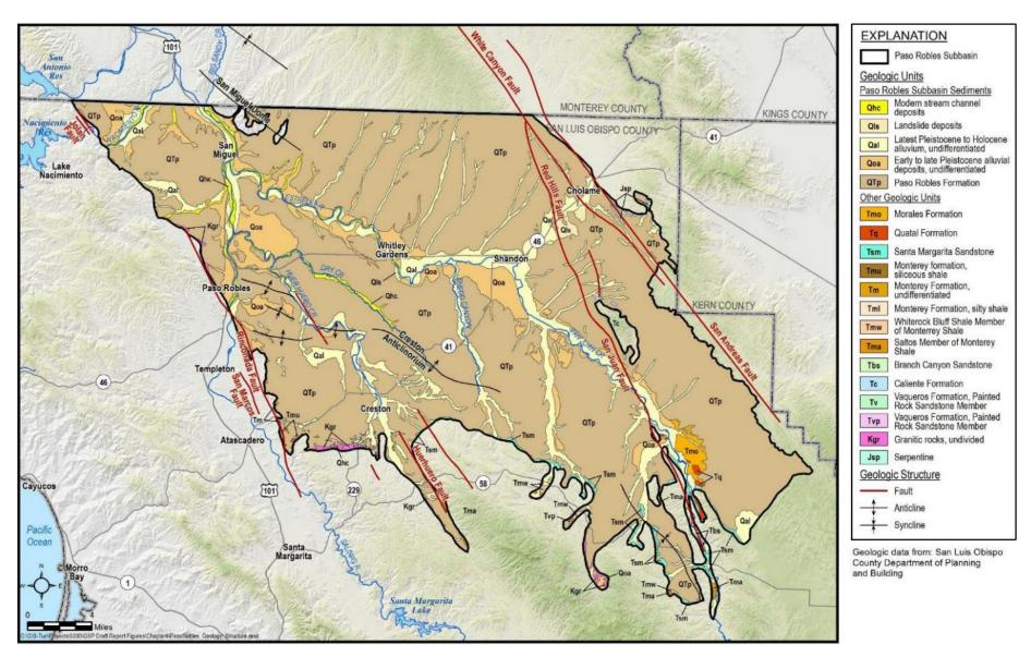
Figure 4-4. Surficial Geology and Geologic Structures
