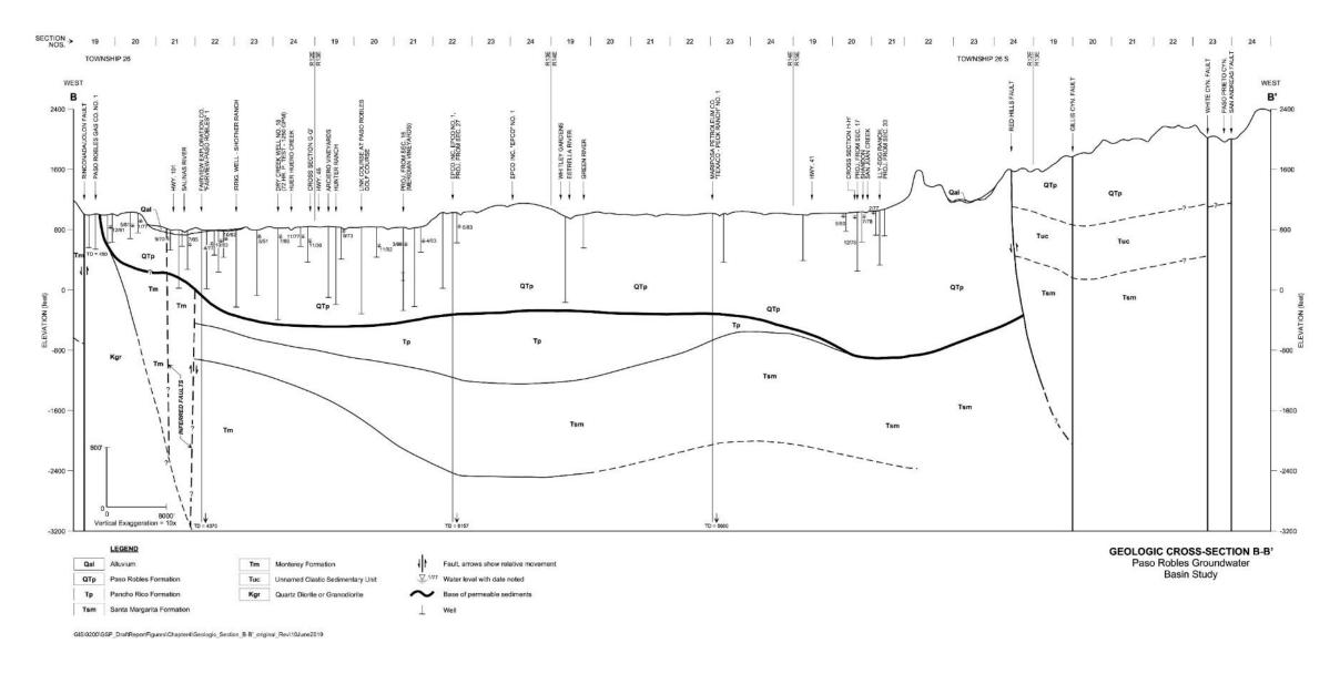
Figure 4-7. Geologic Section B-B'
