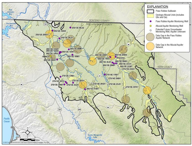
Figure 7-3. Data Gaps in the Groundwater Level Monitoring Well Network
