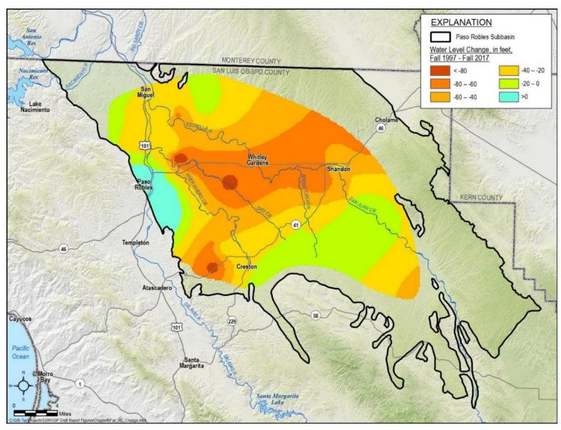
Figure 5-8. Paso Robles Formation Aquifer Change in Groundwater Elevation – Fall 1997 to Fall 2017
