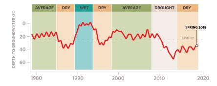
Figure 3. Example seasonality and interannual variability in depth to groundwater over time. Selecting one point in time, Spring 2018, such as groundwater characterize conditions in GDEs fails to capture what groundwater conditions are necessary to maintain the ecosystem status into the future so adverse impacts are avoided.
