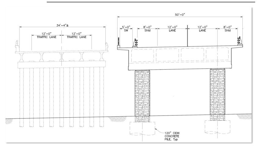
Figure 4 - Cross section views comparing existing and proposed bridge
