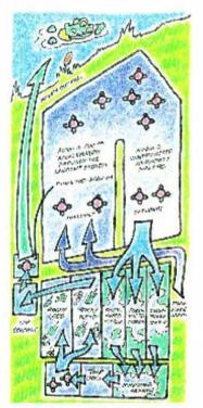
he artificial marsh-rock/reed filter system is essentially a controlled natural process for the secondary and tertiary treatment of wastewater following primary treatment in the oxidation pond, according to project engineering consultant Tim Mader of Mader-Miers Engineering, Inc. in Lafayette.
