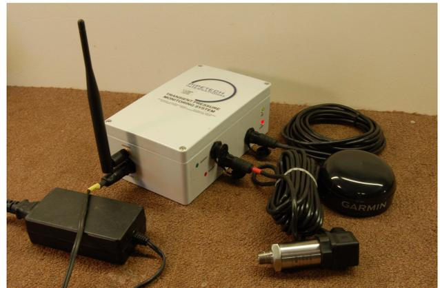
Figure 4 – TP-1 Transient Pressure Monitoring System
