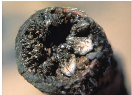
QMs clog pipes and intake structures causing severe damage that requires heavy annual maintenance
