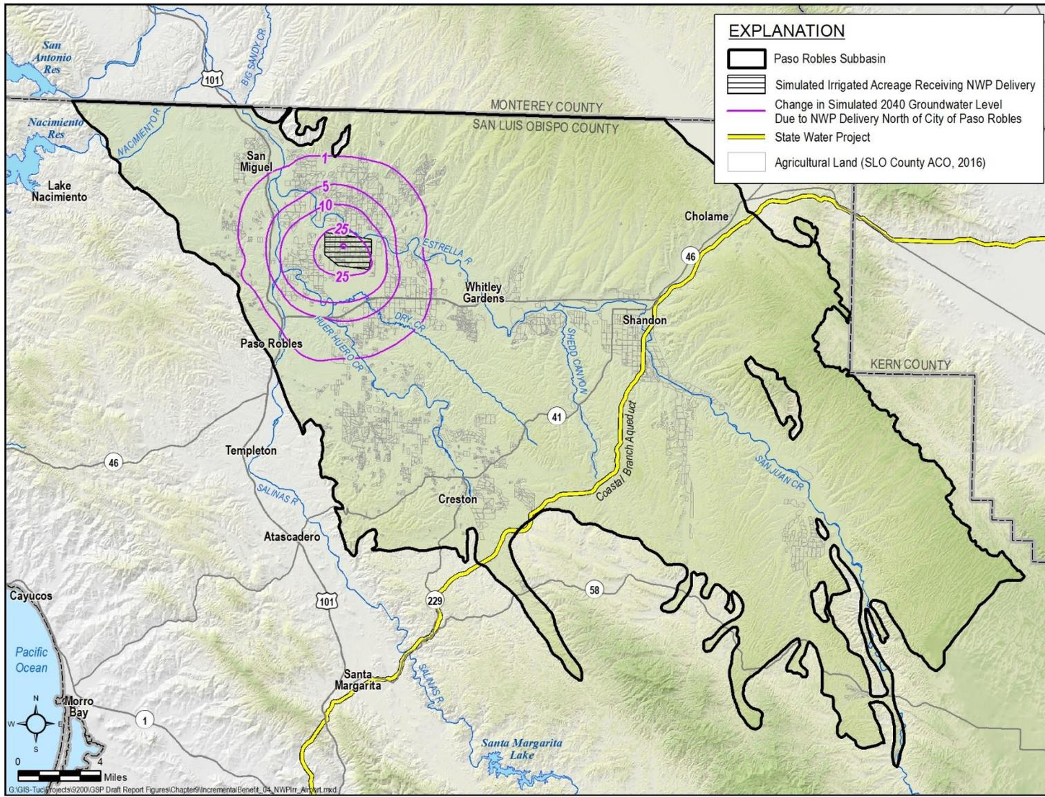
Figure 9-12. Groundwater Level Benefit from NWP Delivery North of City of Paso Robles
