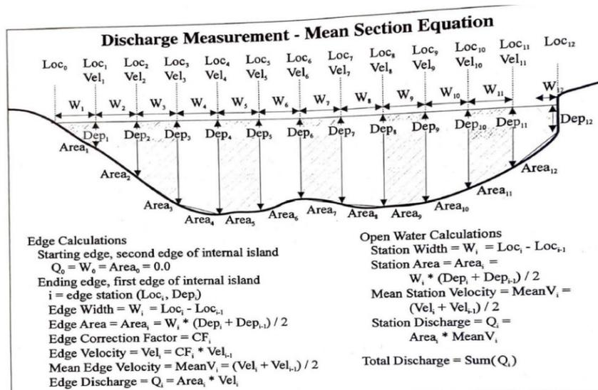
Figure 8 – Discharge Measurement - Mean Section Equation
