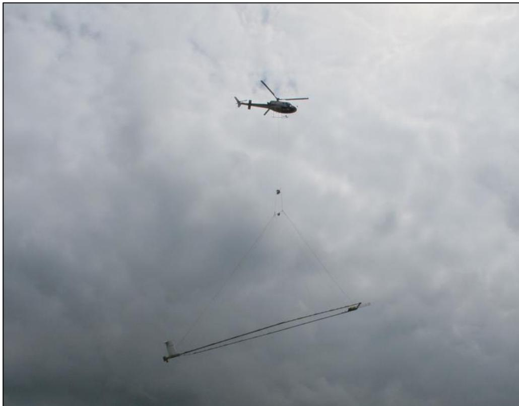
**Figure 3: SkyTEM312M Airborne unit.**
