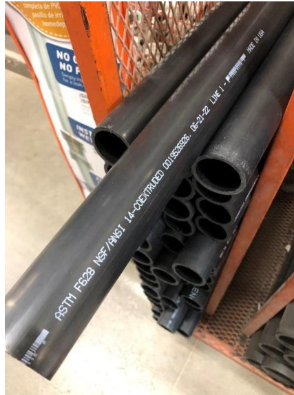
Non-potable/wastewater black PVC pipe
