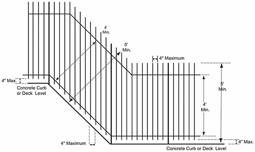
**Figure 31B-4 Perpendicular Fencing Dimensions on Sloping Ground**
