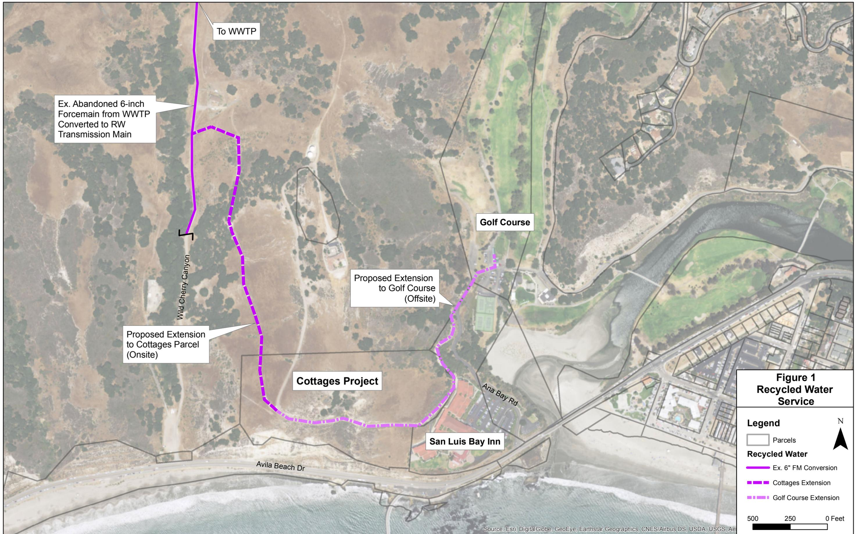
Ex. Abandoned 6-inch Forcemain from WWTP Converted to RW Transmission Main
