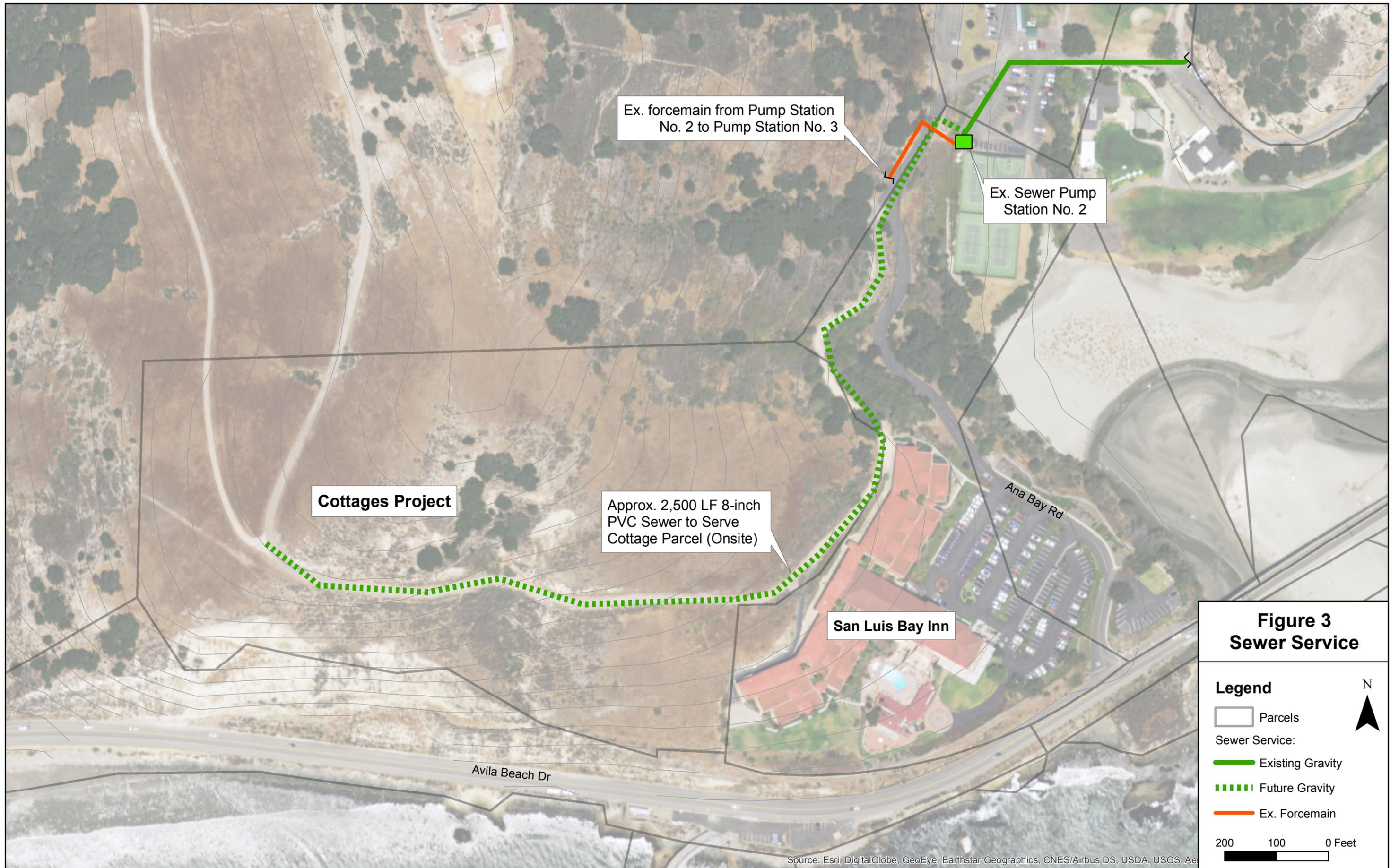
Ex. forcemain from Pump Station No. 2 to Pump Station No. 3
