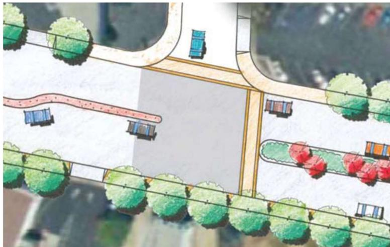
Additionally, pedestrian striping (or special pavers) across the intersection is included to better define the pedestrian areas. However, in order to reduce potential conflicts and assist traffic flow, pedestrian crossings are confined to the northern and eastern sides of the intersection. There is sufficient right-of-way (ROW) width to allow plantings in the raised median east of 10th Street.
