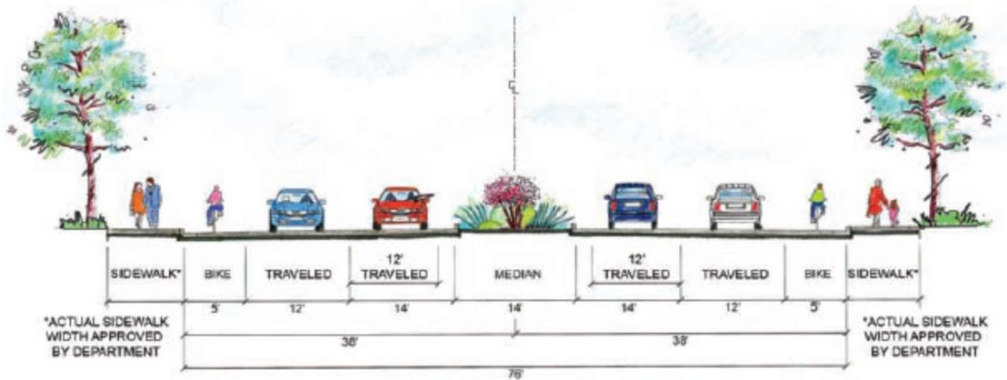
A raised median provides three main functions: 1) restrict the unobstructed movements and control the turning movements, 2) provide traffic calming by narrowing the roadway, causing traffic to slow down, and 3) provide an opportunity for plantings and other hardscape improvements, enhancing the streetscape and the visual character of Los Osos Valley Road.
