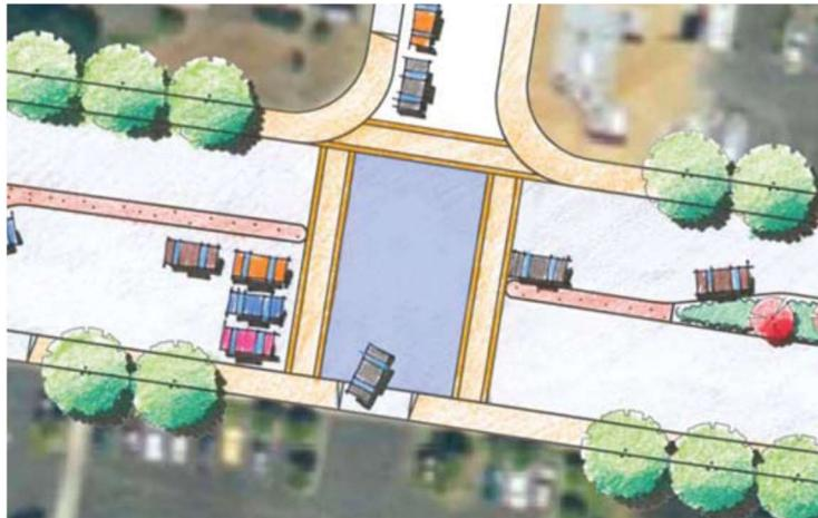
The signal would also be synchronized with the other traffic signals along Los Osos Valley Road for traffic flow timing and enhanced peak hour movement. The Corridor Study recommends adding pedestrian striping (or special pavers) across the intersection to better define the pedestrian areas.
