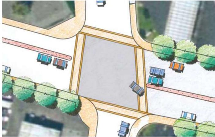
The signal would also be synchronized with the other traffic signals along Los Osos Valley Road for traffic flow timing and enhanced peak hour movement. Additionally, pedestrian striping (or special pavers) across the intersection is included to better define the pedestrian areas. There is insufficient right-of-way (ROW) width to allow plantings in the raised median nearest the intersection.
