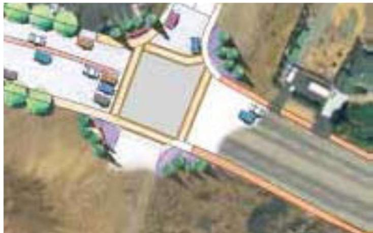
The Corridor Study recommends pedestrian striping (or special pavers) across the intersection to better define the pedestrian areas on all sides of the intersection except the east side. In addition, sidewalks should tie into the proposed trail heading southeast down Los Osos Valley Road.
