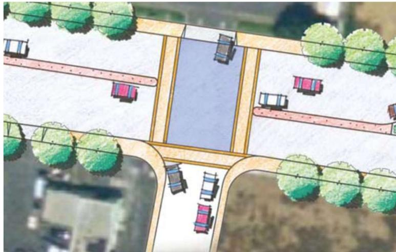
A traffic signal is not included under either option, but a set of “STOP” signs is recommended in both options to control traffic onto Los Osos Valley Road. Los Osos Valley Road traffic would not be subject to a “STOP” sign under any option.
