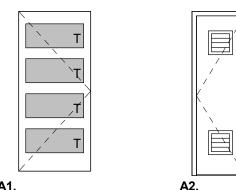
**EXTERIOR - ENTRY -EXTERIOR** -SOLID CORE WOOD **VENTED WATER HEATER DOOR**
