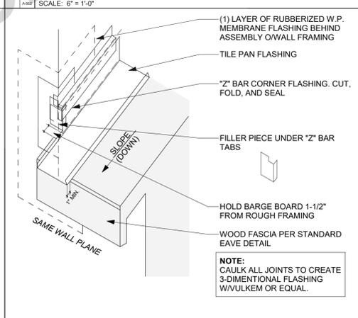
**12 ROOF TO WALL TYP. FLASHING 2**
