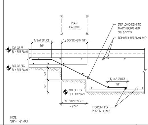
STEP IN CONCRETE SLAB ON GRADE
