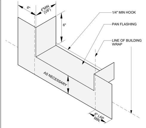
**23 FLASHING PAN @ DOOR THRESHOLD**
