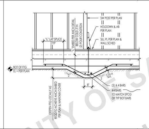
SLAB ON GRADE EDGE AND SUBGRADE PREP
