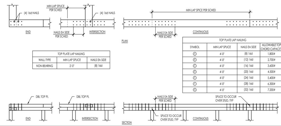
51 DBL TOP PLATE SPLICE NAILING 227-01-C102-1463 NTS 32
