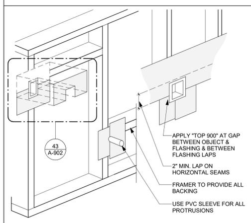
**43 FLASHING - PROTRUSIONS**
