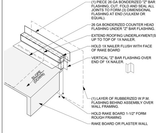
**13 ROOF TO WALL TYP. FLASHING 3**
