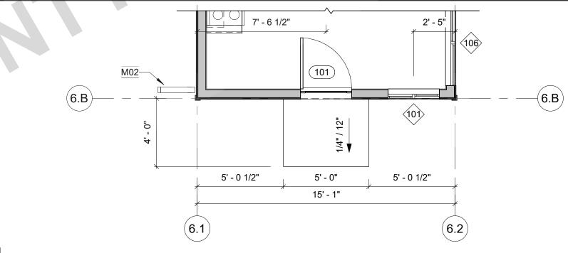
**GROUND FLOOR PLAN - NO FRONT PORCH OPTION** A1-201 A6-101 SCALE: 1/4" = 1'-0'
