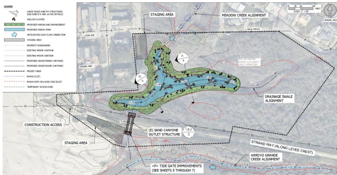
Figure 16. Meadow Creek Lagoon Enhancement Project - 30% Design - Plan.
