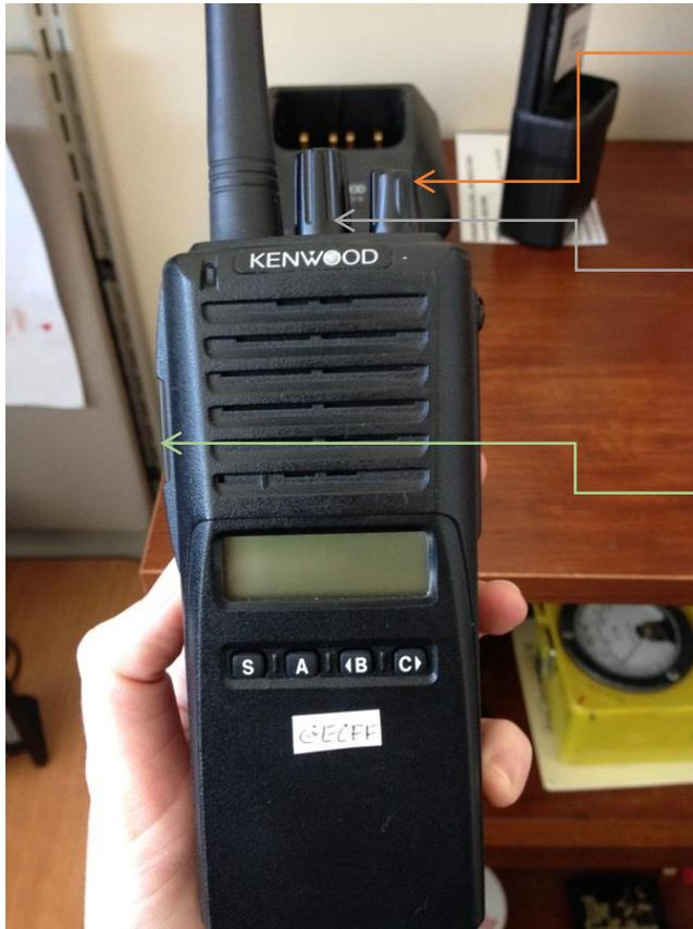
**Step 1: Turn Radio On** – Turn the far right button on.
