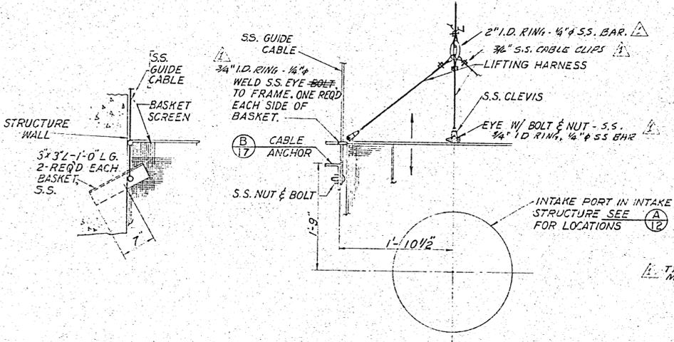
GUIDE CABLE ANCHOR DETAIL (B) NO SCALE
