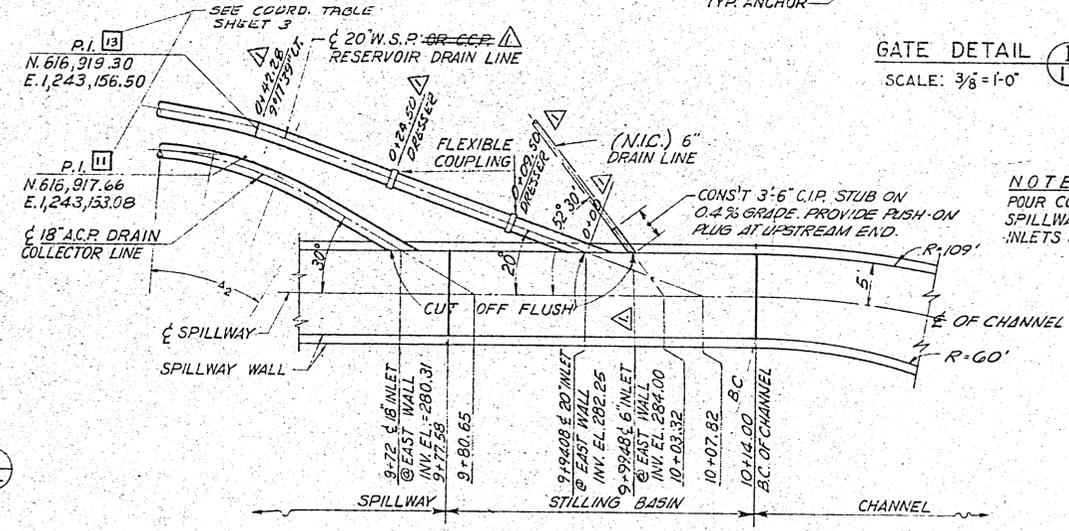
SPILLWAY INLETS DETAIL (J) SCALE: 1" = 10'
