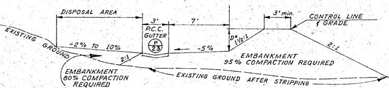
**PERIMETER CHANNEL EMBANKMENT SECTION E**
