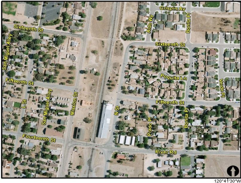
The project will fence existing RR right of way north of 14th Street, install sidewalk along a portion of River Road and install gated pedestrian crossing at 16th Street.
