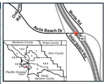
The project will construct a single lane roundabout at the intersection of Avila Beach Drive and Shell Beach Road and the northbound offramp/southbound on and off ramps of the US 101 interchange. A Park & Ride lot and RTA bus stop will also be constructed.
